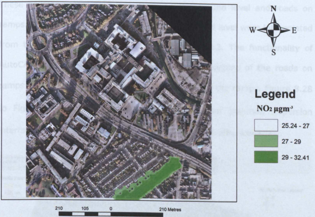
Figure 8.27 Contour Map of 2021 30 metres-height Annual Mean \text{NO}_2 Concentrations in the Dunkirk AQMA for the Effective Alternative NET Phase 2 Traffic Scenarios
