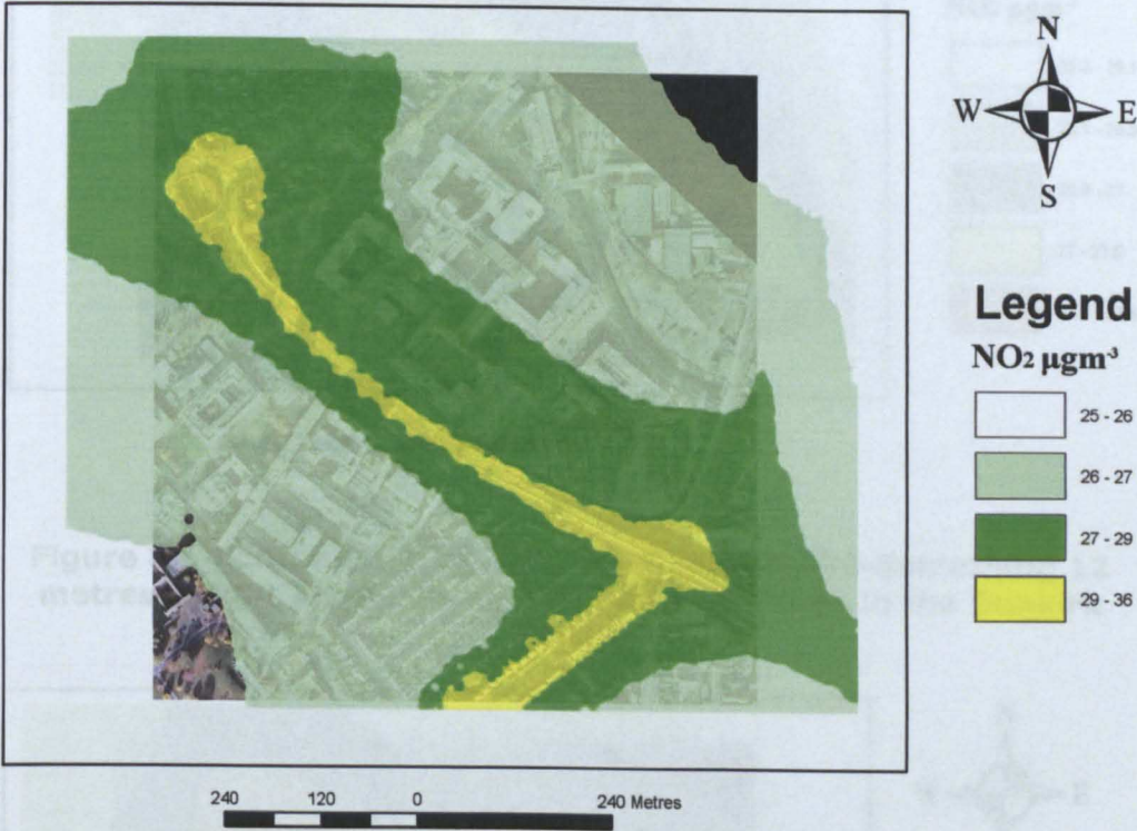
Figure 8.4 Contour Map of 2021 Do-Minimum/Do-Something 6 metres-height Annual Mean NO 2 Concentrations in the Dunkirk AQMA
