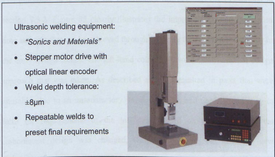
Figure 83: Implemented ultrasonic welding equipment
