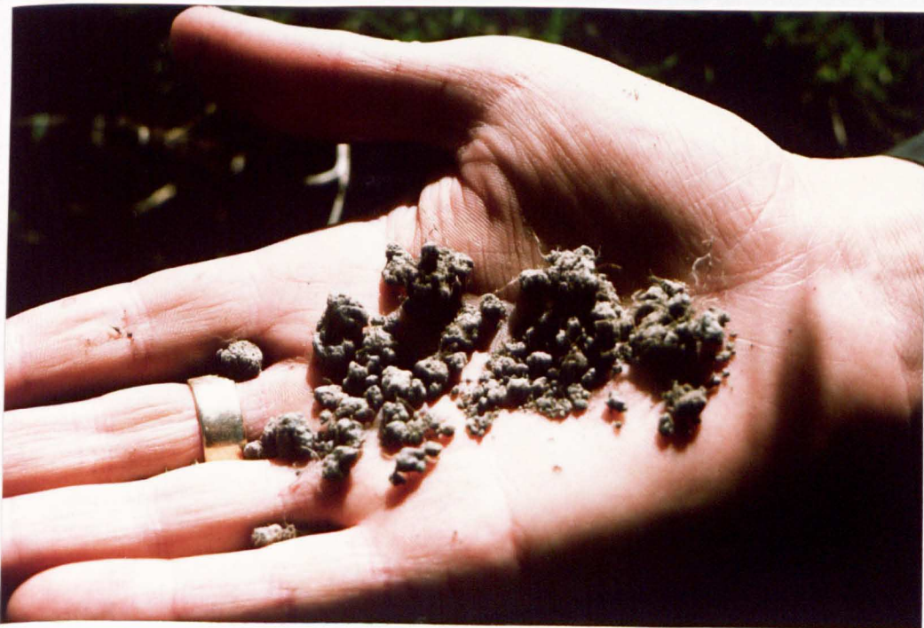
Plate 3.7 Non-Cohesive Aggregates of Cohesive Bank Materials
