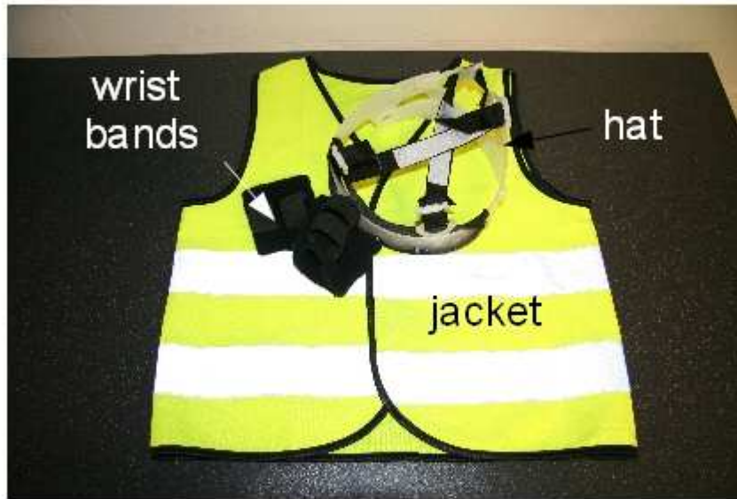
Figure 2.8: Picture showing the motion gear which the child wears over their own clothes. The motion trackers are attached to the motion tracking gear using industrial Velcro.
