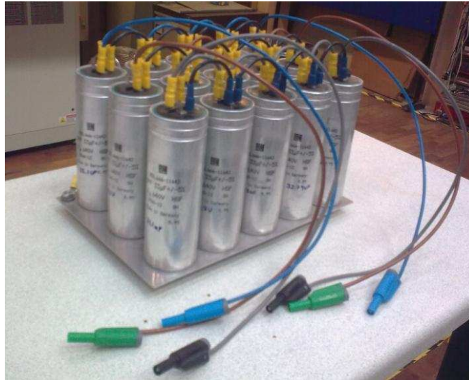
Figure 7.17 Photographs of the series AC capacitors
