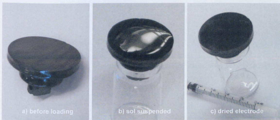
Fig. 6.2. Sol casting electrode fabrication.
