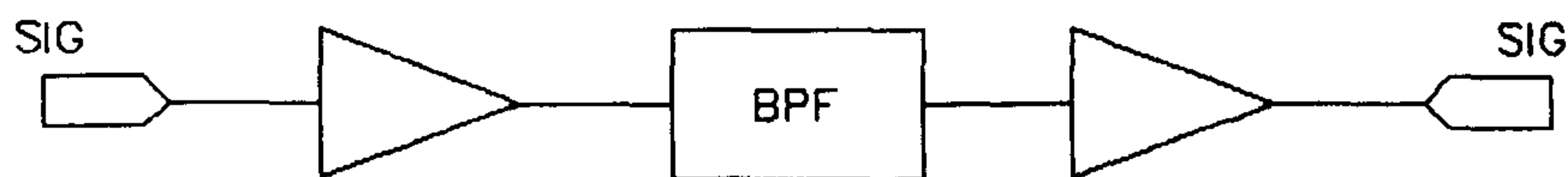
Figure 9: Block diagram of signal conditioning card.
