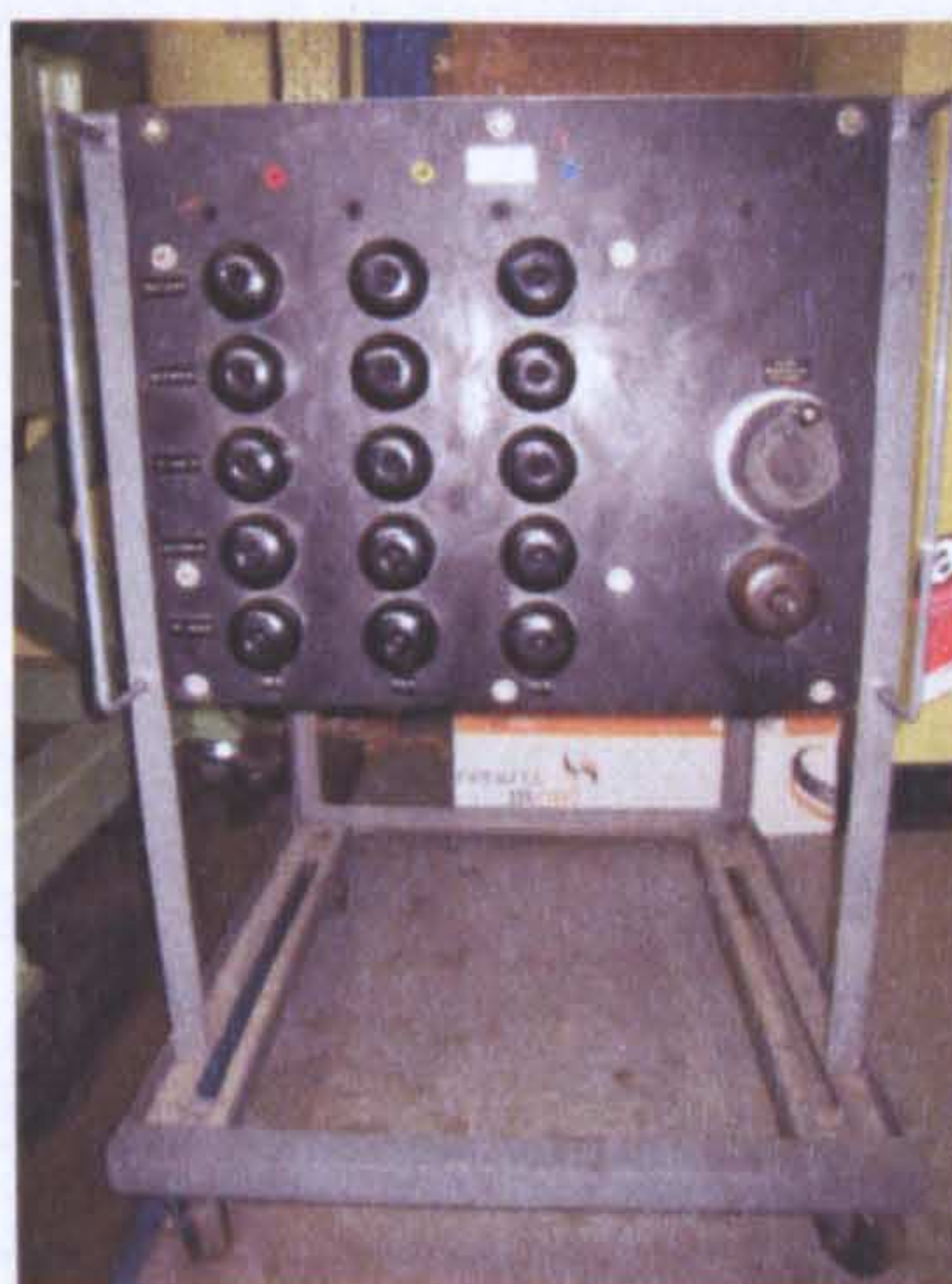
Figure 5.7: The resistive load
