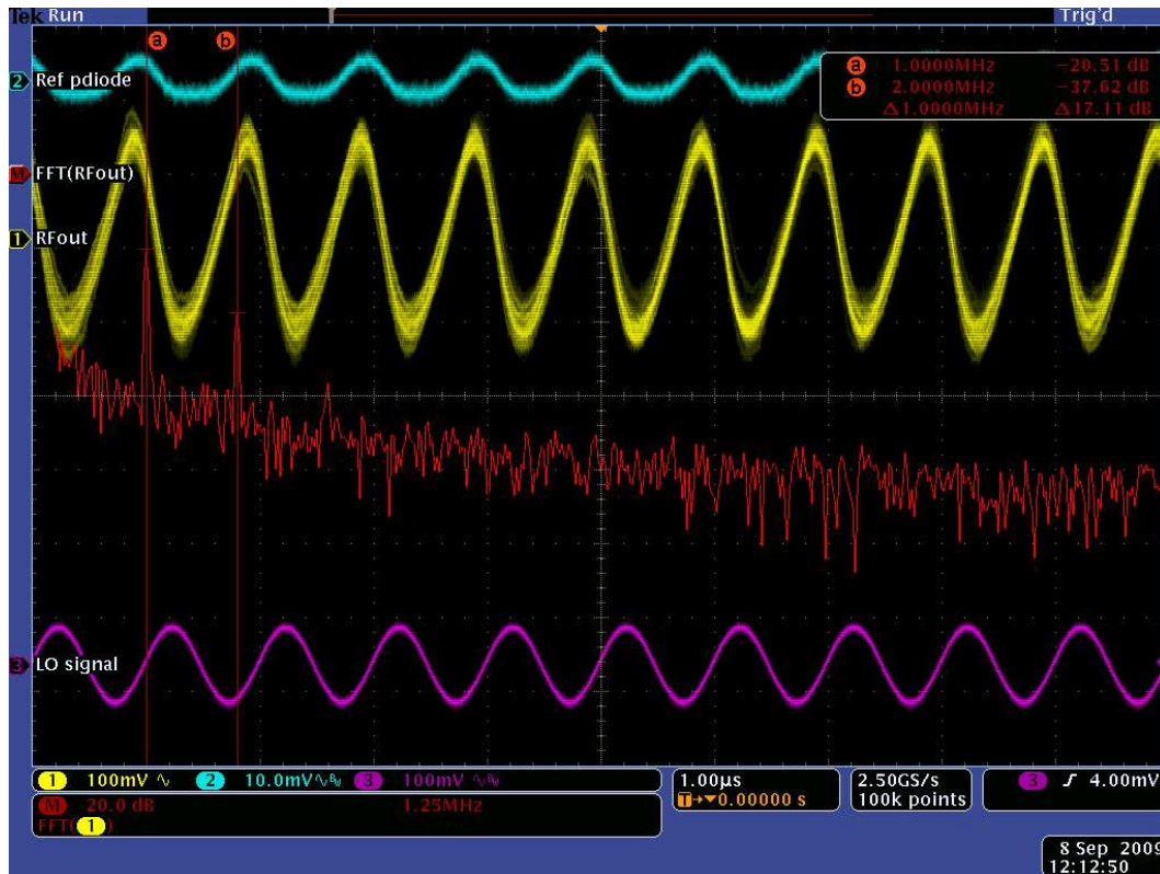
Figure 4.42: Response of MLCv6 to a 1MHz RF signal. Tunebias = 0nA in this case. This is compared with the LO signal, the signal from the reference PD-36A photodiode. The FFT of the RF signal is also shown.
