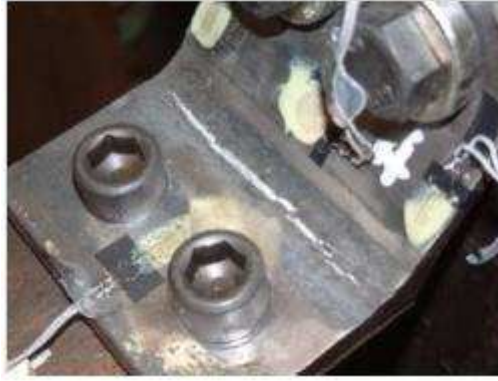
Figure 2.15 : Top view of the fracture due to low cycle fatigue (Elghazouli et al., 2009)
