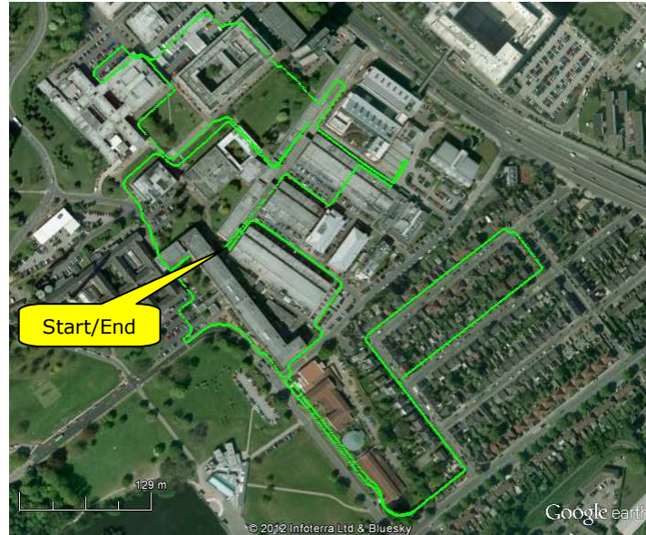
Fig. 8.26: Low-cost PNS/ZUPT with MPA trajectory solution
