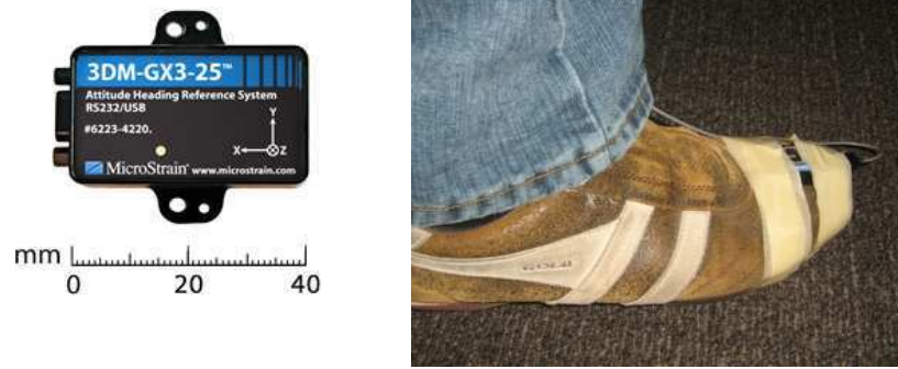
Fig. 5.3: The 3DM-GX3-25 IMU from MicroStrain (left) and mounted on a shoe (right).
