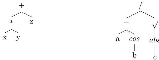
Figure 5.1: General arithmetic expressions as parse trees, (left) x \cdot y + z , (right) \frac{a - \cos(b)}{\sqrt{|c|}} .
