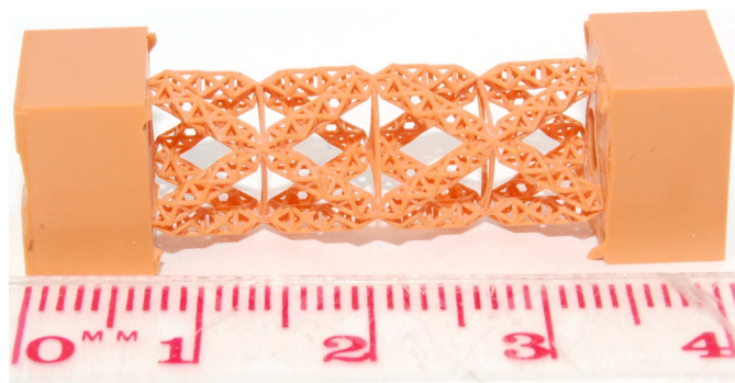
Figure 5.6: The generation-2 frame. The final frame was built without the top tetrahedron and with a plate attached to both top and bottom to allow reliable compression tests to be undertaken.
