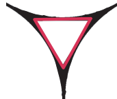
Figure 7.41: Area of the largest equilateral triangle that fits in the 2D shape of the MN.
