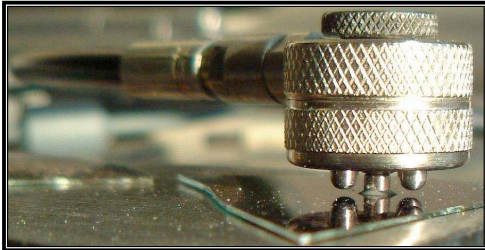
Figure 2.15 Pull off test developed by DFD ® Instruments (Source: DFD ® Instruments n.d.)
