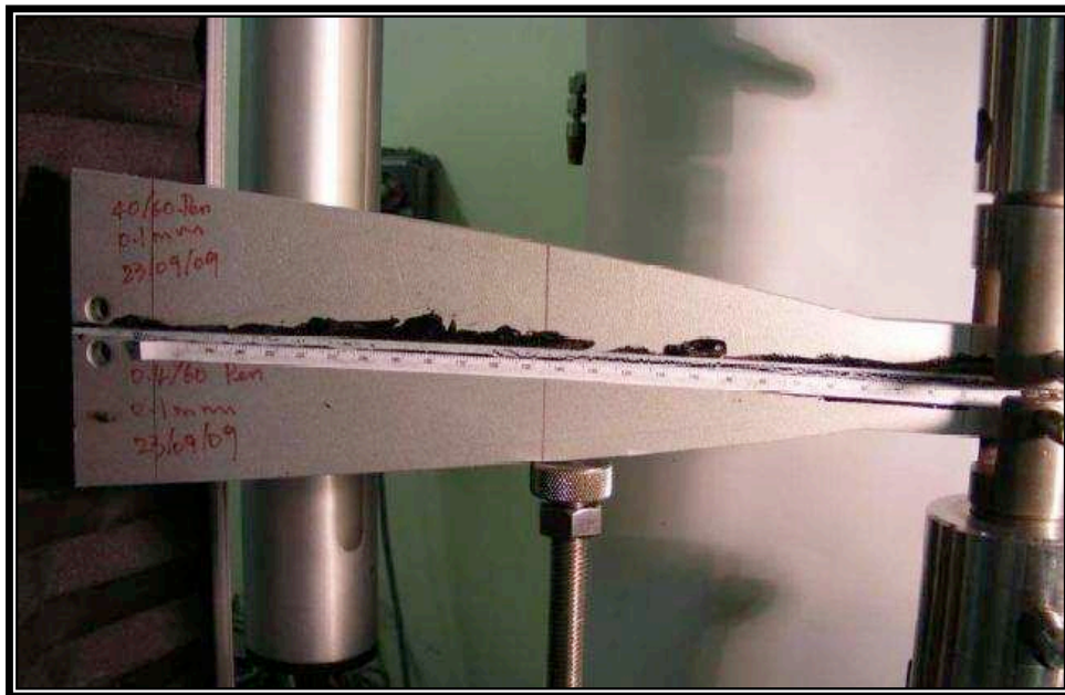
Figure 2.23 TDCB test using bitumen as adhesive materials and aluminium alloy as substrates (Source: Cui et al. 2010)
