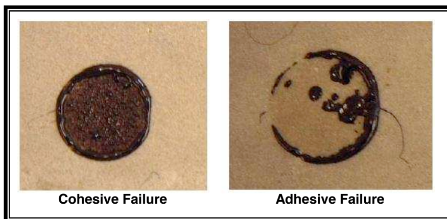
Figure 2.40 Types of failure of tested specimens using PATTI 110 (Source: Kanitpong & Bahia 2003)
