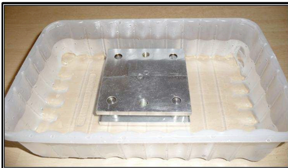
Figure 6.16 Specimen immersed in container filled with water
