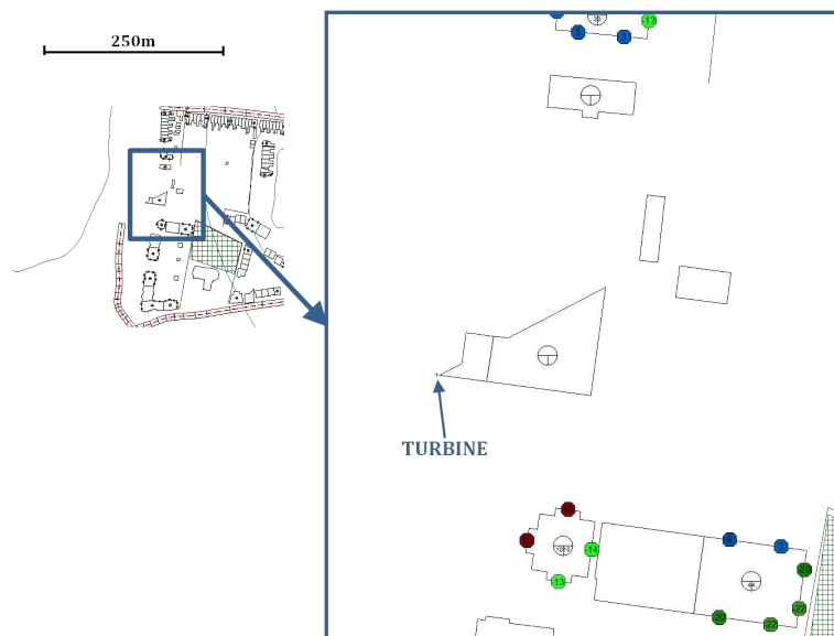
Figure D.2.8: Map of installation (f) showing area topography and sound pressure levels at building facades close to the turbines
