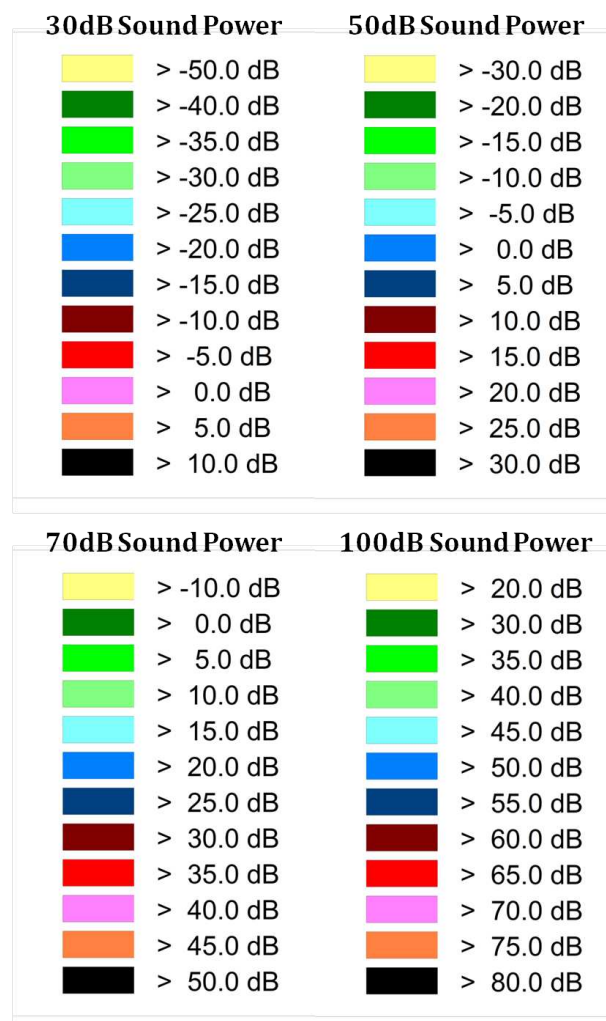
Figure D.1.1: Colour palettes for sound maps produced using CadnaA software package for a 30dB, 50dB, 70dB and 100dB sound power point source
