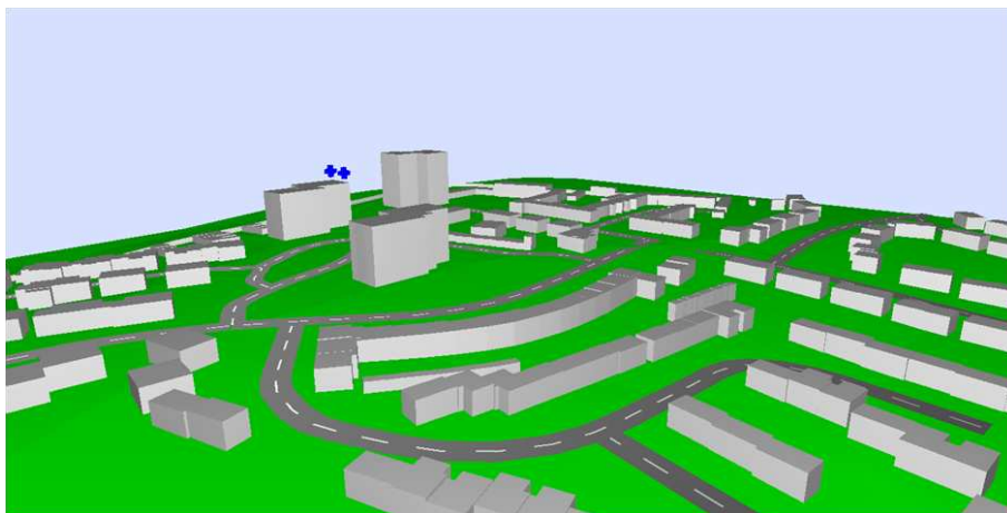
Figure 2.2.5: 3D View of installation (d) showing wind turbines as point sound sources marked as blue crosses
