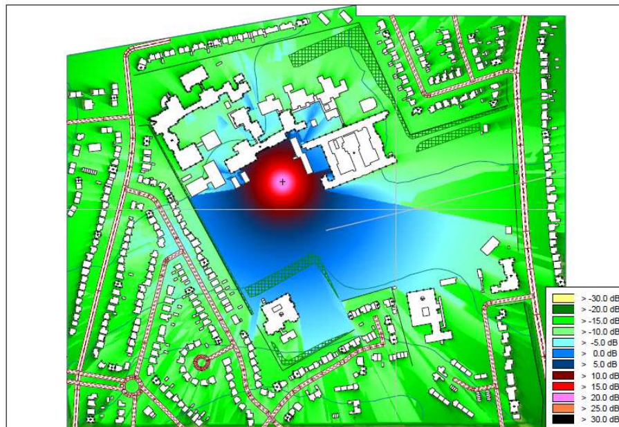
Figure 2.2.7: Sound map for installation (c) showing attenuation of sound from a 50dB turbine
