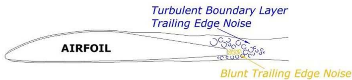
Figure 1.2.4: Turbulent Boundary Layer Trailing edge Noise and Blunt Trailing Edge Noise Mechanism
