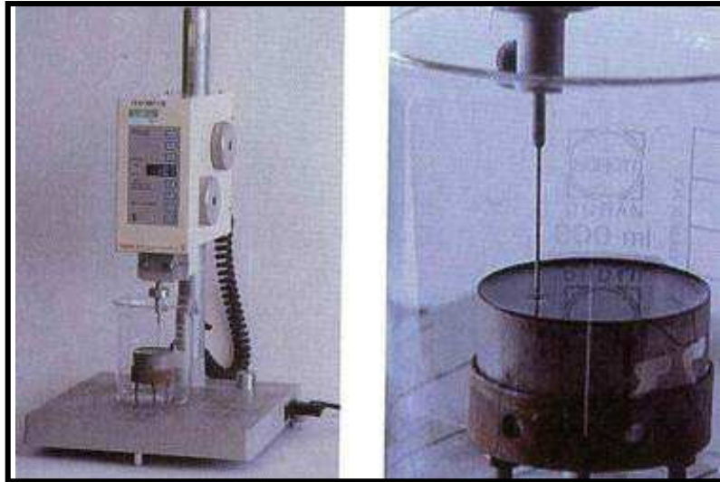
Fig. 2.1: The penetration test [Read and Whiteoak, 2003]
