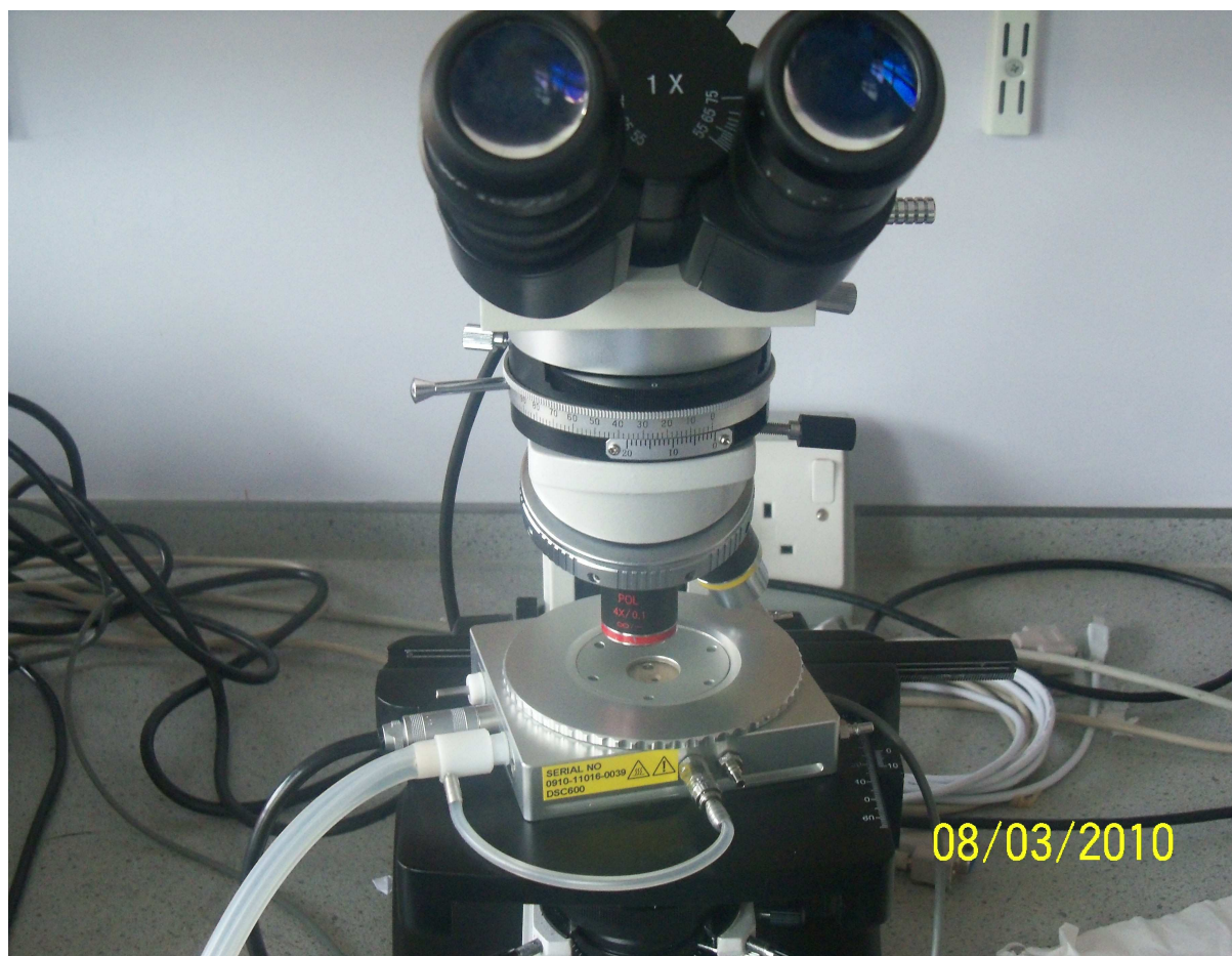
Figure 9: Microscope heating stage (Linkam) mounted on the rotating stage of a polarizing light microscope in the Laboratory of Biophysics and Surface Analysis, School of pharmacy, University of Nottingham
