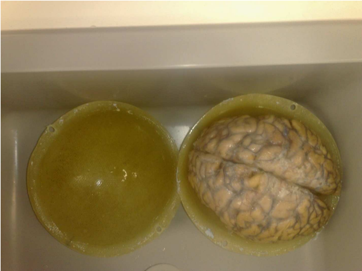
Illustration of a post-mortem brain in the purpose designed MRI compatible holder
