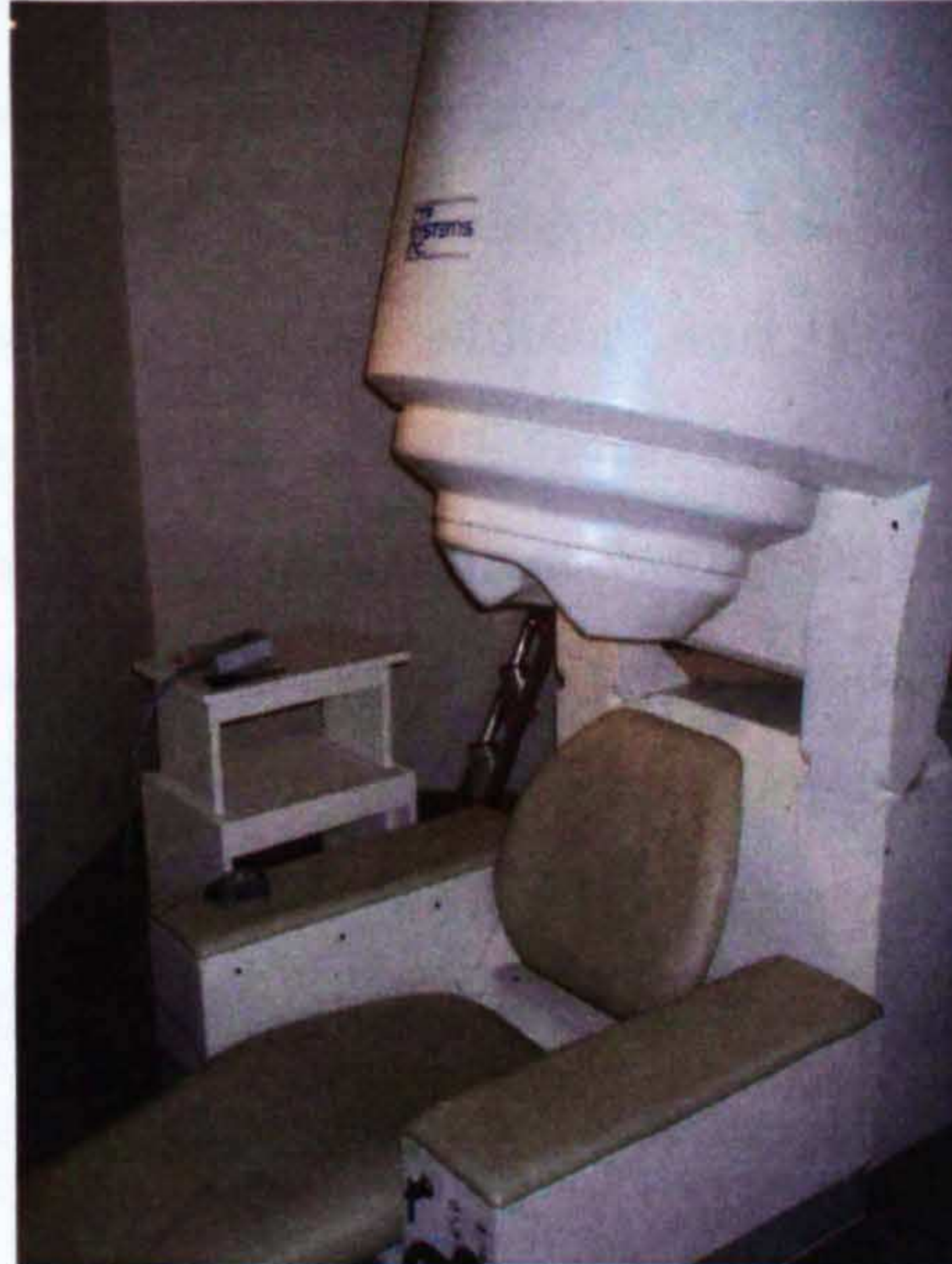
Figure 4.7: The MEG system manufactured by CTF Systems Inc. , used in this study.
