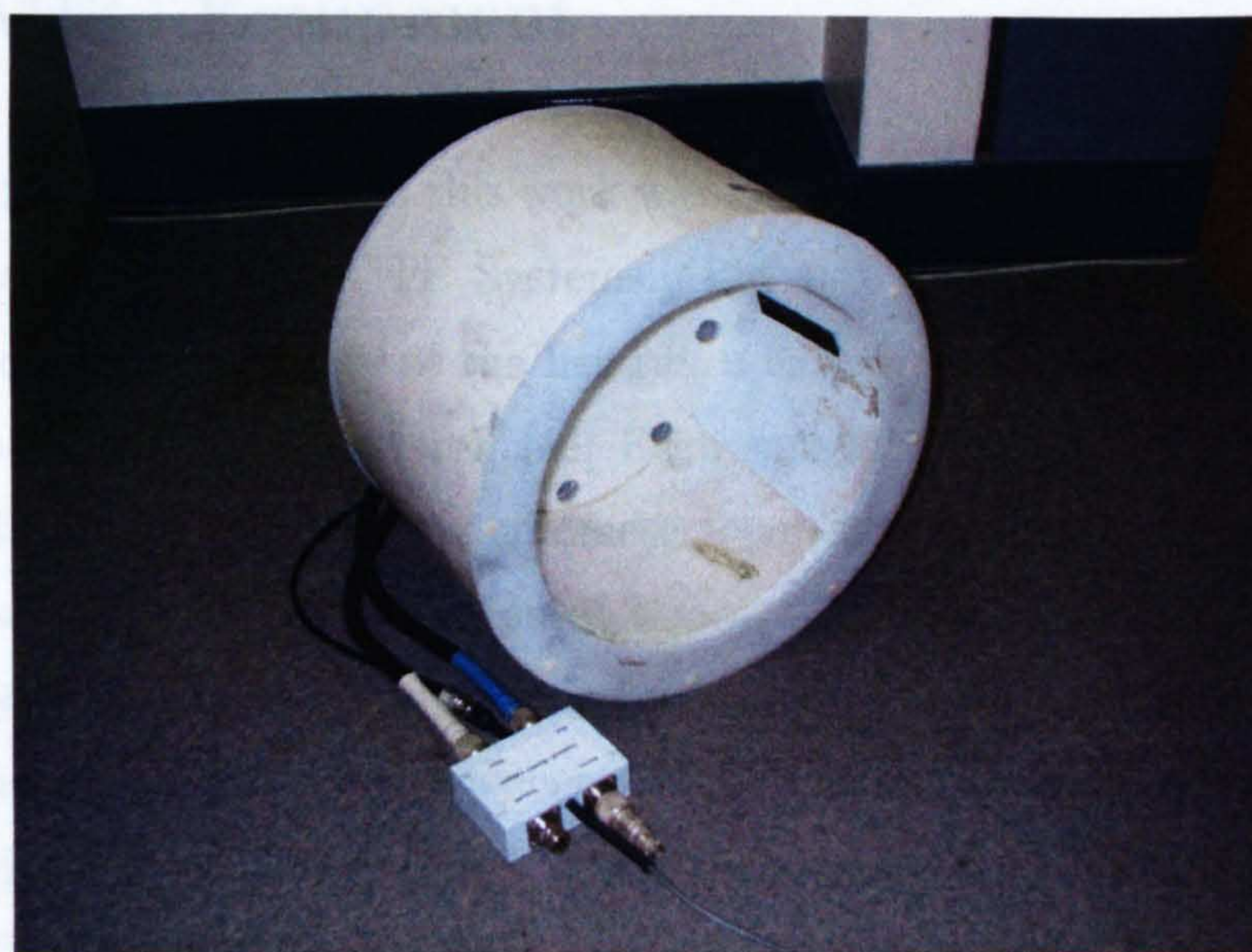
Figure 4.6: The TEM coil, of 26.5 cm in diameter and 23 cm in length, manufactured by MR Instruments Inc. used in this study.
