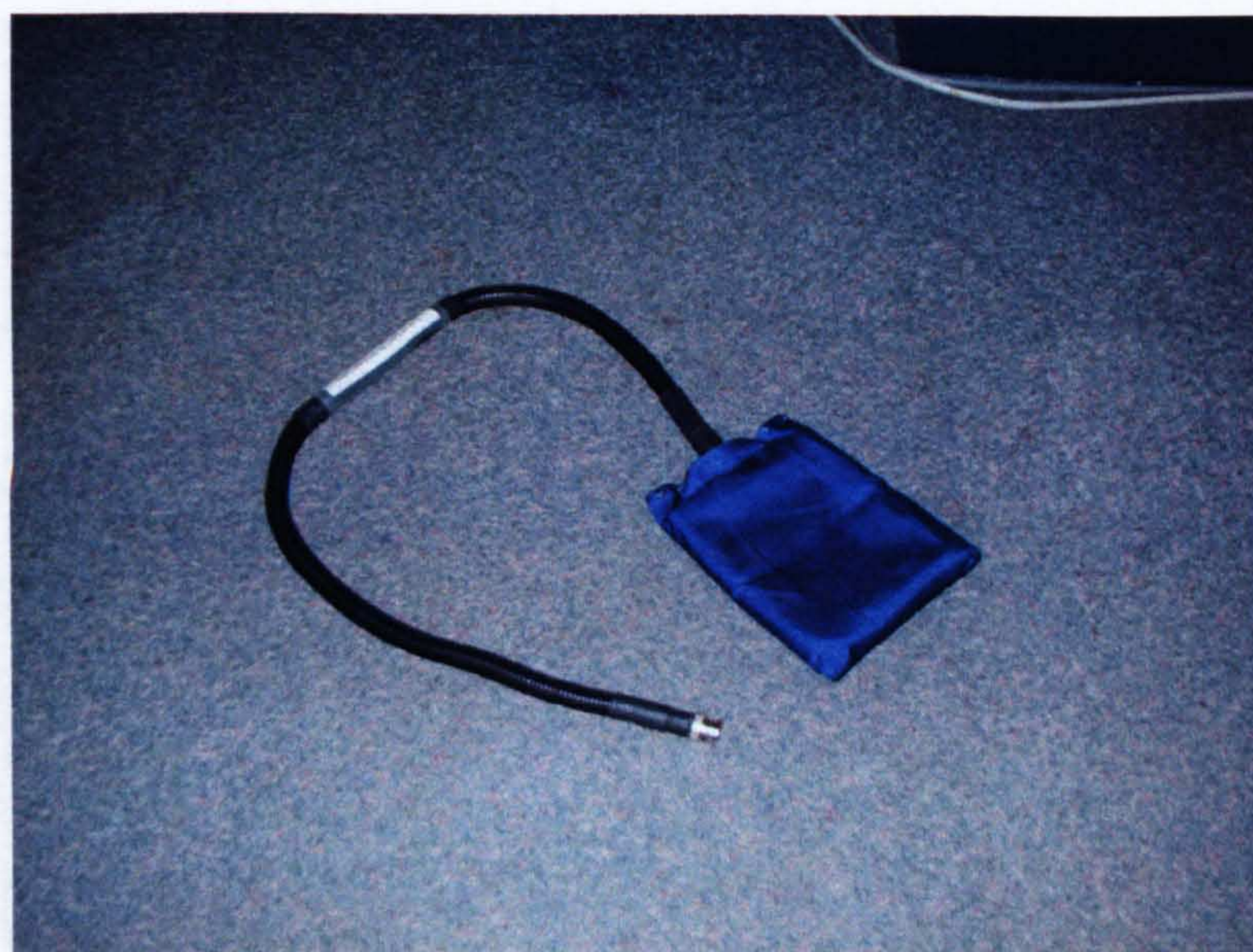
Figure 4.4: The surface coil, of 9 cm in diameter, manufactured by MR Instruments Inc. used in conjunction with TEM coil in this study.
