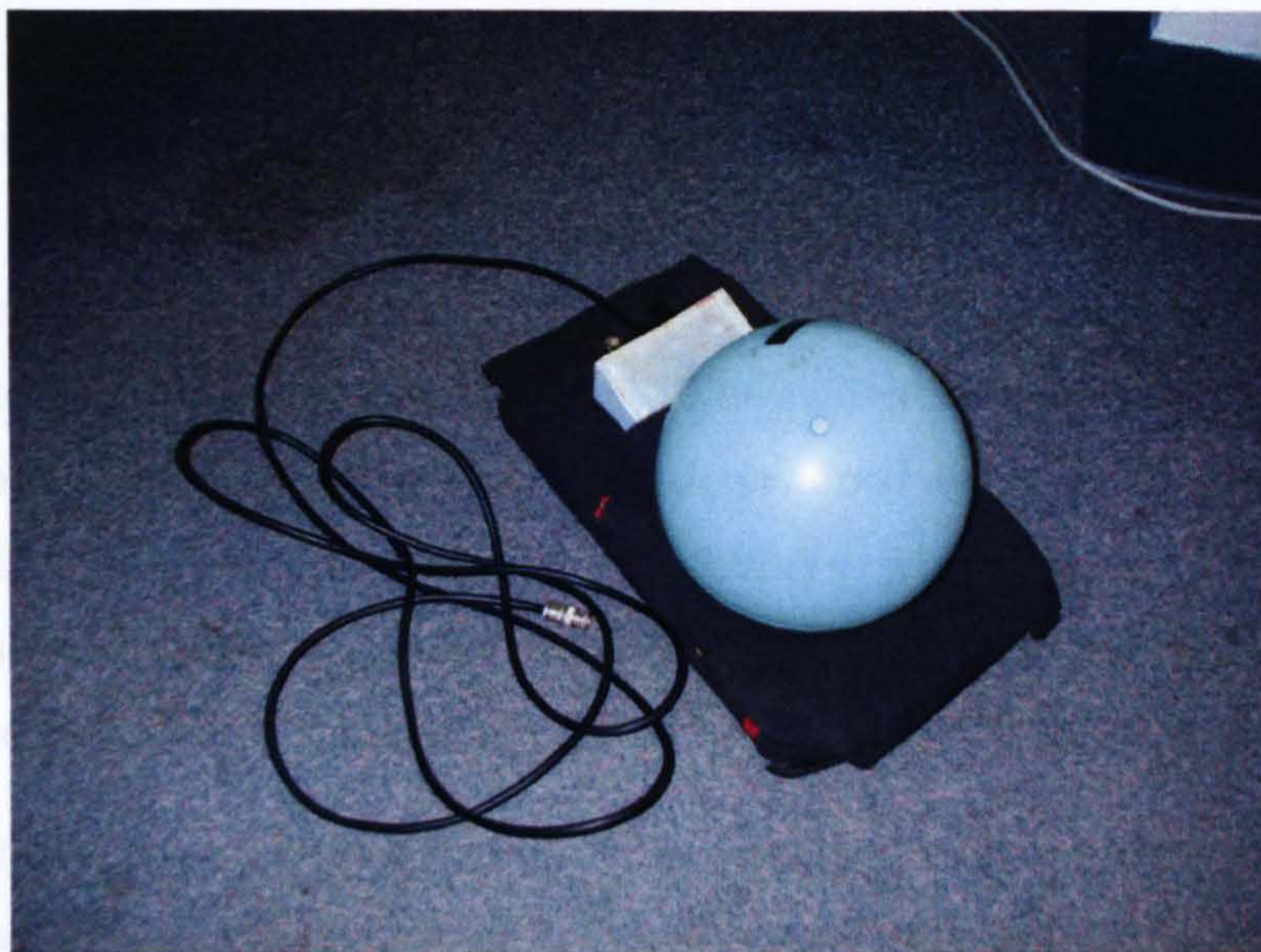
Figure 4.5: The home made surface coil, of 14 cm in diameter, used in this study and a phantom.
