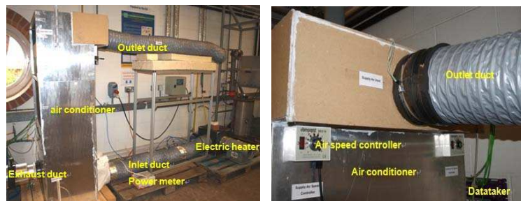
Fig. 4-10 The photograph of dew point cooler test system in laboratory
