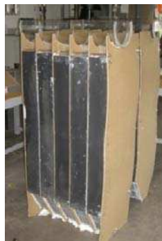
(g) Finished heat/mass exchanger
