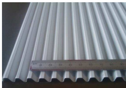
Fig. 5-16 Real guide geometry of corrugated sheet
