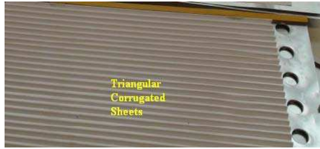
Fig. 4-7 The corrugated sheets for supporting channels of heat exchanger
