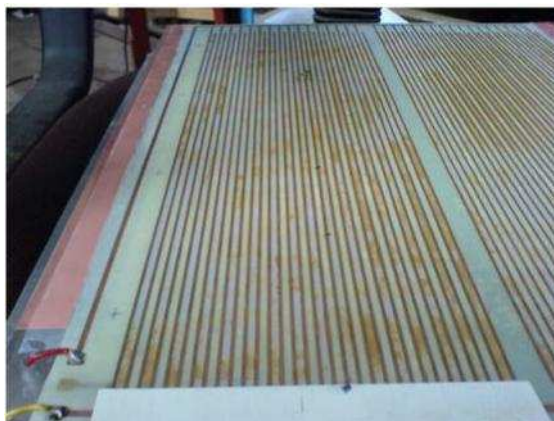
Figure 10.1.1. Detail of burnthrough of electrode sheet after the PEF = 50Hz experiment. Note discoloured regions and pitted areas of the Mylar material in plasma regions.
