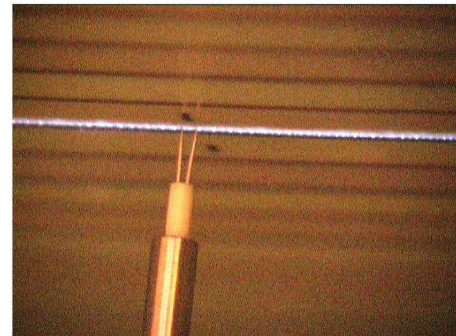
Figure 5.3.11. Colour enhanced images of the asymmetric plasma actuator at: a) t \approx 40\text{ms} ; b) t \approx 80\text{ms} after plasma initiation. Hot wire shown in figure and the prongs have 1.25mm spacing at their tip. The plasma occurs on both sides of the electrode at initiation (a), although the plasma on the near side appears to be brighter and more uniform. After the first few pulses (b), the plasma formation is entirely one-sided.
