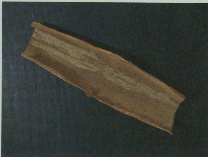
Photograph 4.1: Phosphor Bronze 150µm Screen Mesh Wick
