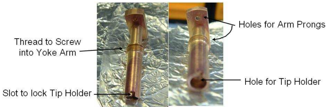
Figure 3.11: Photographs of the Phase Two design tip tool, displaying the hole and slot to hold and lock the tip holder in place. The holes for the UHV arms to manipulate the tip tool and the thread allowing the tip tool to screw into in the yoke arm are also labelled.
