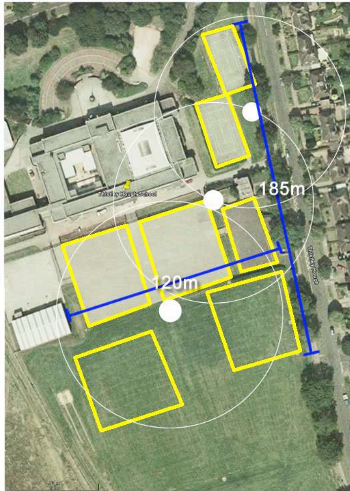
Figure 18: approximate wireless coverage provided by access points in the school grounds for Study 2
