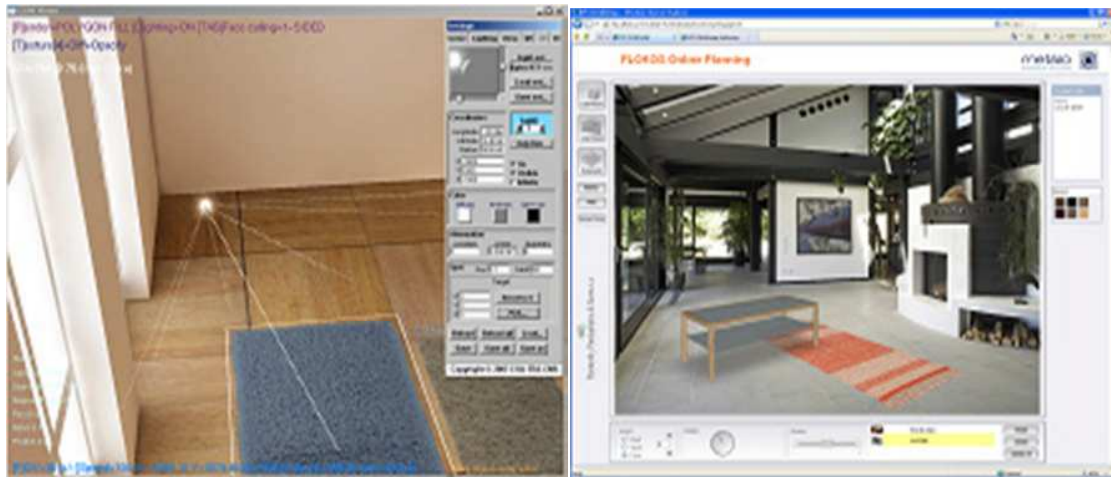
Figure 3-5: Collaborative Product Reviewer - carpet design visualisation tool allowing 3D designs of a carpet to be positioned and superimposed onto a real photo (Bourguignon et al. , 2009)
