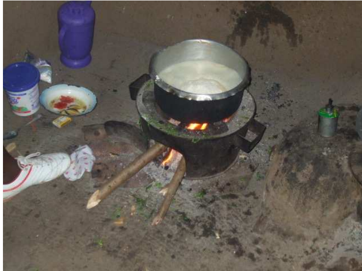
Figure 5.3: The portable Upesi stove
