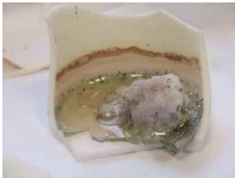
Figure 3.4: The glass produced using raw materials from The Weald (for scale, base of crucible is approximately 4cm in diameter).
