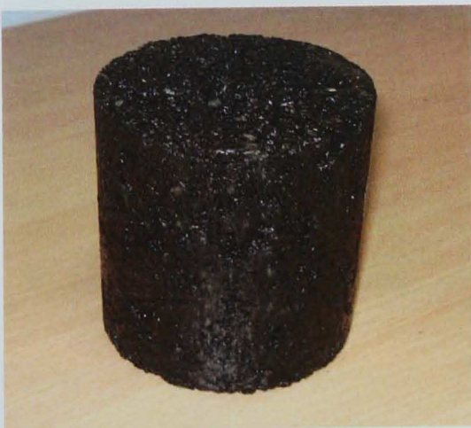
Figure 4.2 Specimen for monotonic compression test
