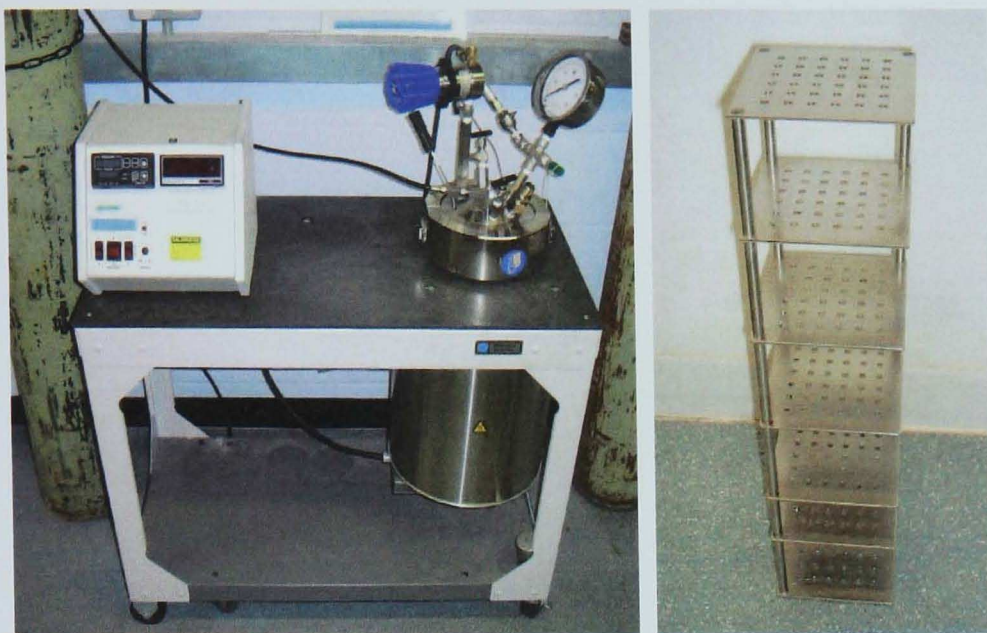
Figure 6.13 (a) Pressure ageing vessel used in the SATS test, (b) specimen rack in vessel
