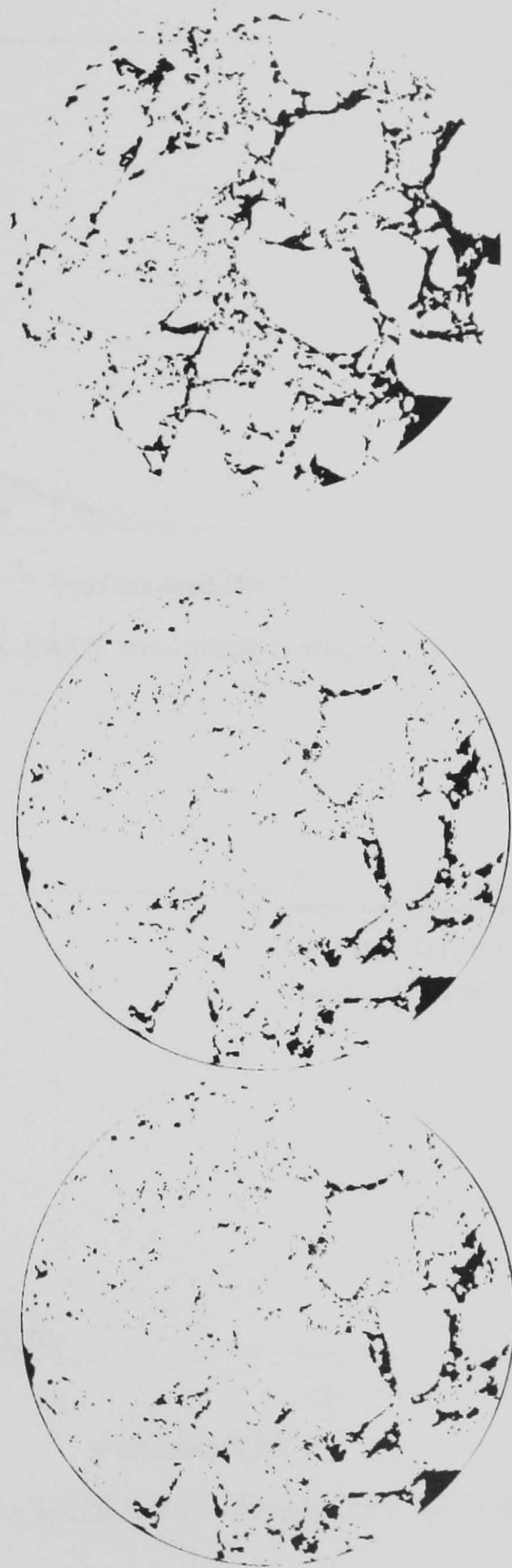
Figure 6.15 Void content from X ray scanning at different stages of SATS test
