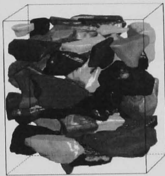
Figure 2.11 3D images of asphalt aggregate (Wang et al. 2004)
