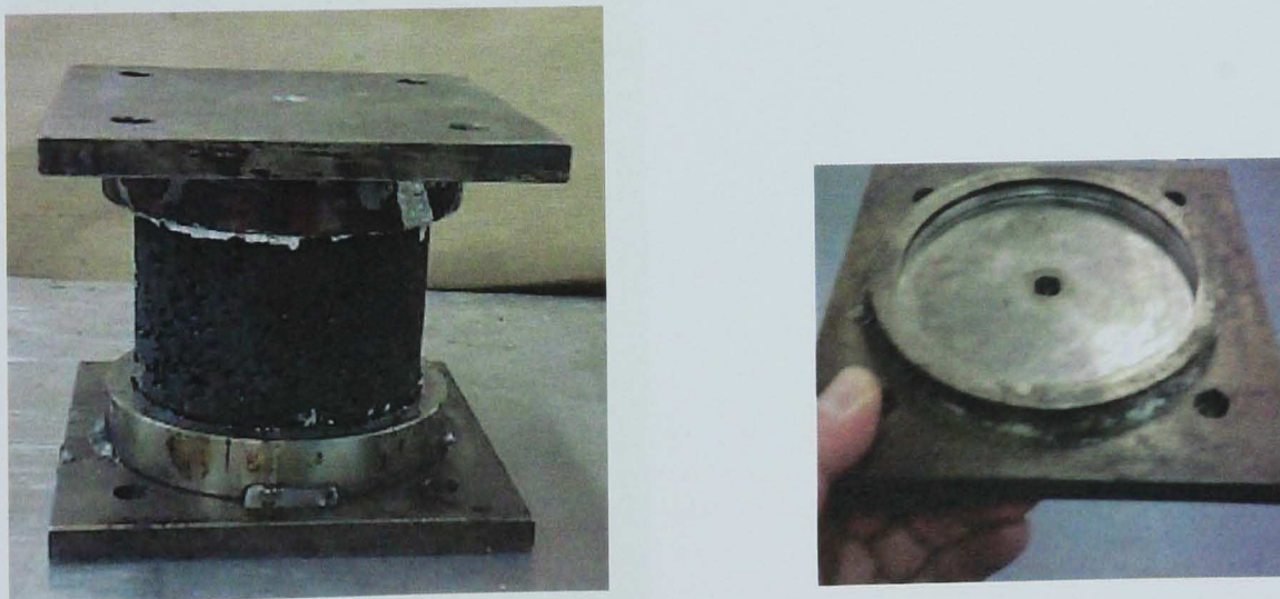
Figure 5.4 a) Specimen glued between in steel plates, b) End plate with 10 mm deep ring with grooves inside
