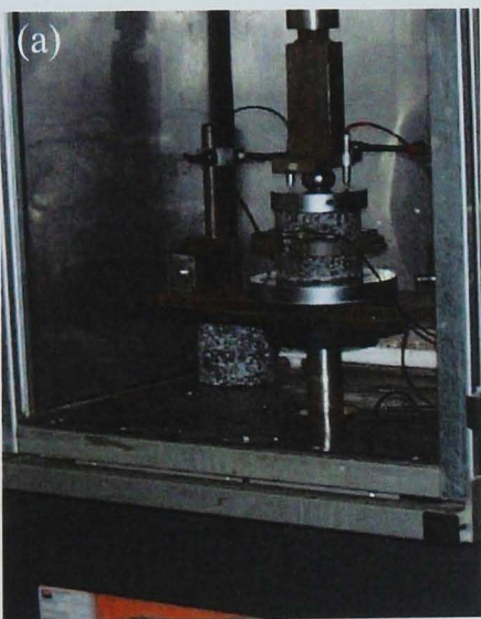
Figure 4.4 a) Sample in monotonic compression test, b) Typical failure of sample in monotonic compression test
