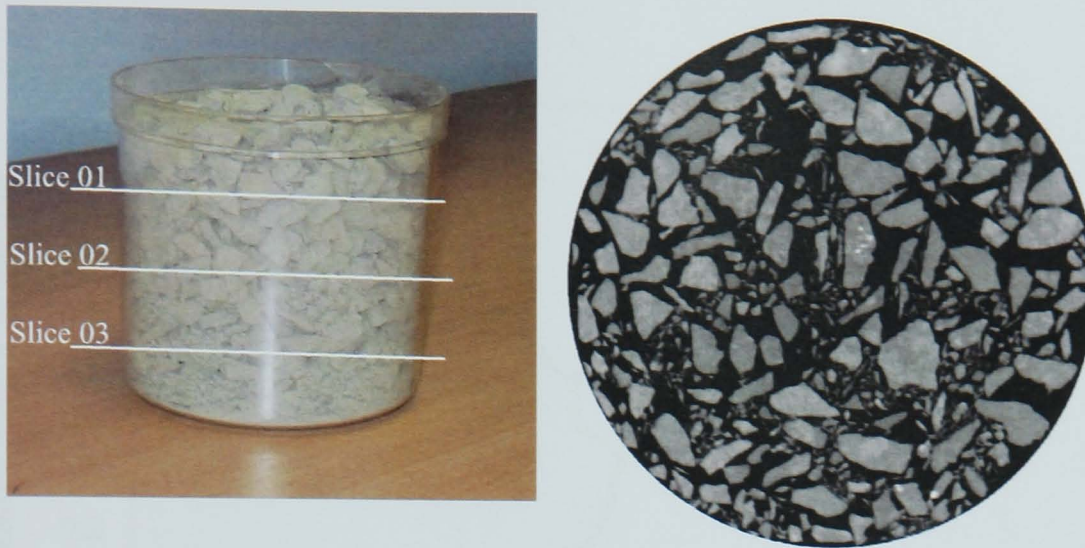
Figure 4.15 a) Aggregate mix for X ray scanning, b) X ray image of aggregate without binder
