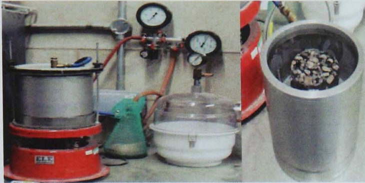
Figure 6.3 Laboratory setting for saturating the specimen
