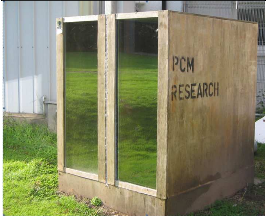
Figure 8.5: Outdoor PCM test box with 2 identical chambers
