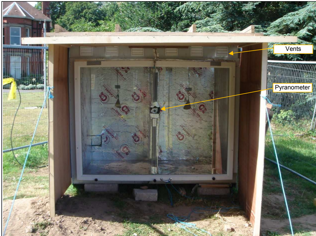
Figure 8.35: Picture of the outdoor rig at the School of the Built Environment, University of Nottingham
