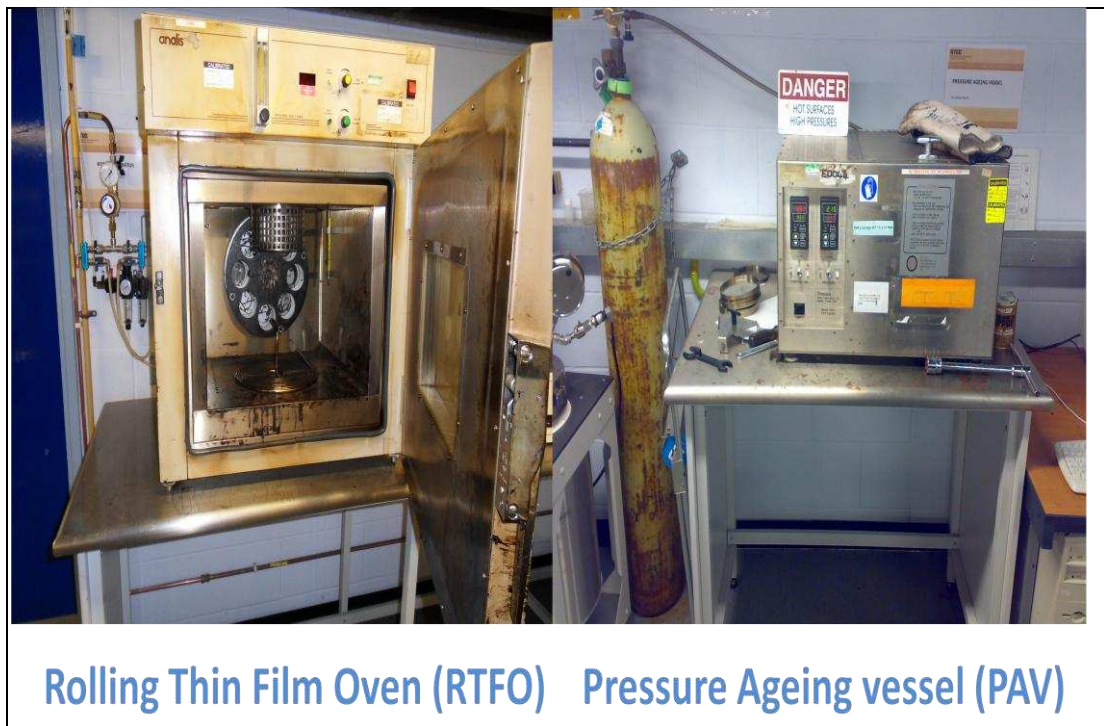
Figure 4.4: Facilities for Bulk Binder Ageing
