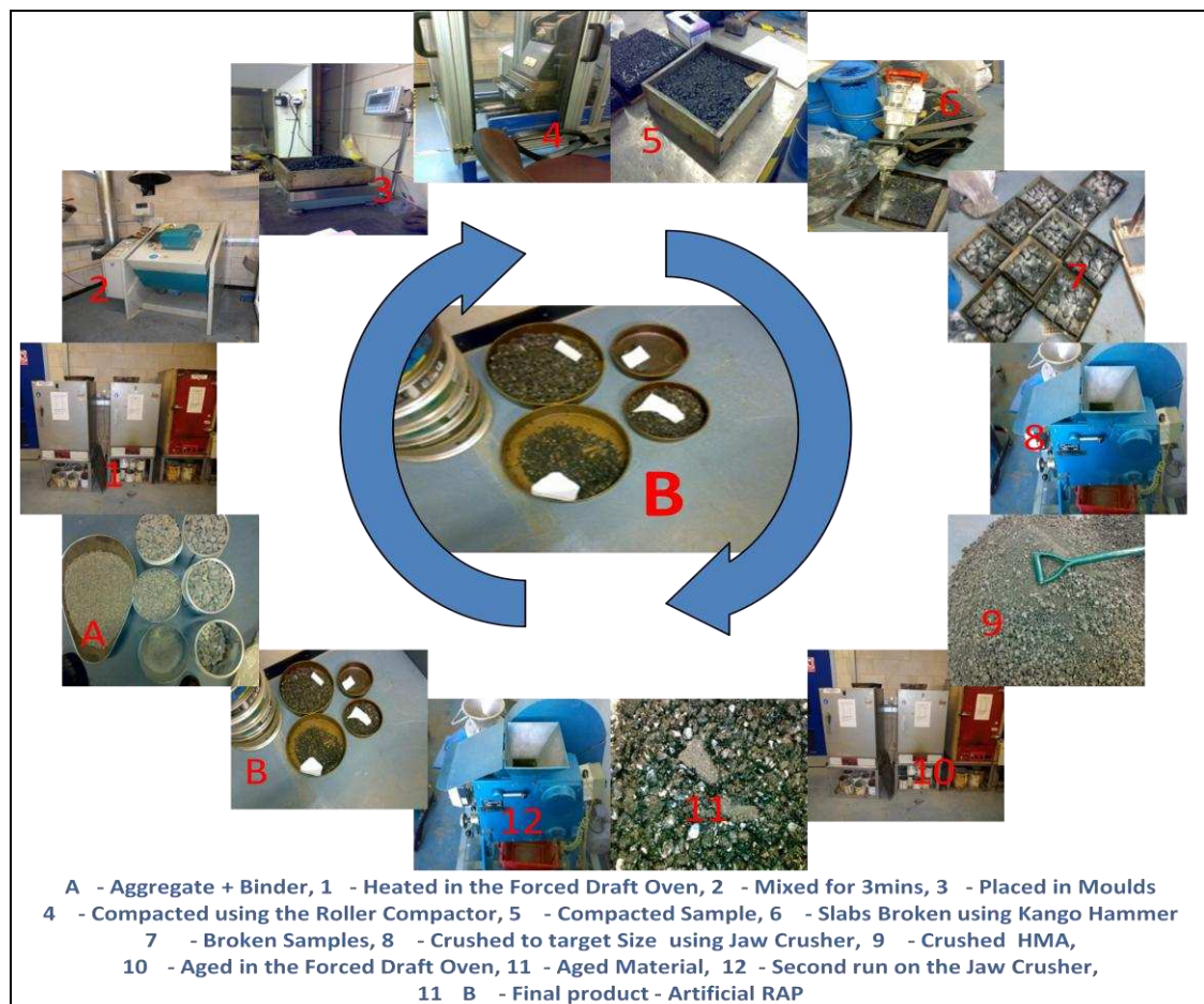
Figure 4.2: Laboratory Procedure for the Production of Severely Aged RAP
