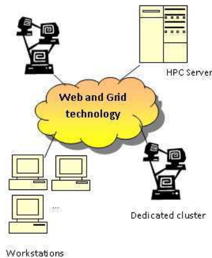
FIGURE 2.2: Computational grid architecture: internet-based interconnection of heterogeneous and distributed individual workstations, dedicated clusters, high performance computing (HPC) servers and clusters of distributed PCs (Desktop PC Grid)
