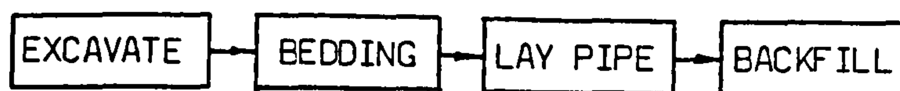
Figure (5.3.1) Sequence of work of the Trenching operation
