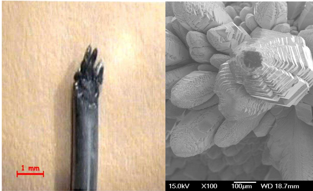
Figure 5.2b: Silver sulphide crystals grown on the apex of a silver wire (left) and a SEM image of some silver sulphide crystals (right).
