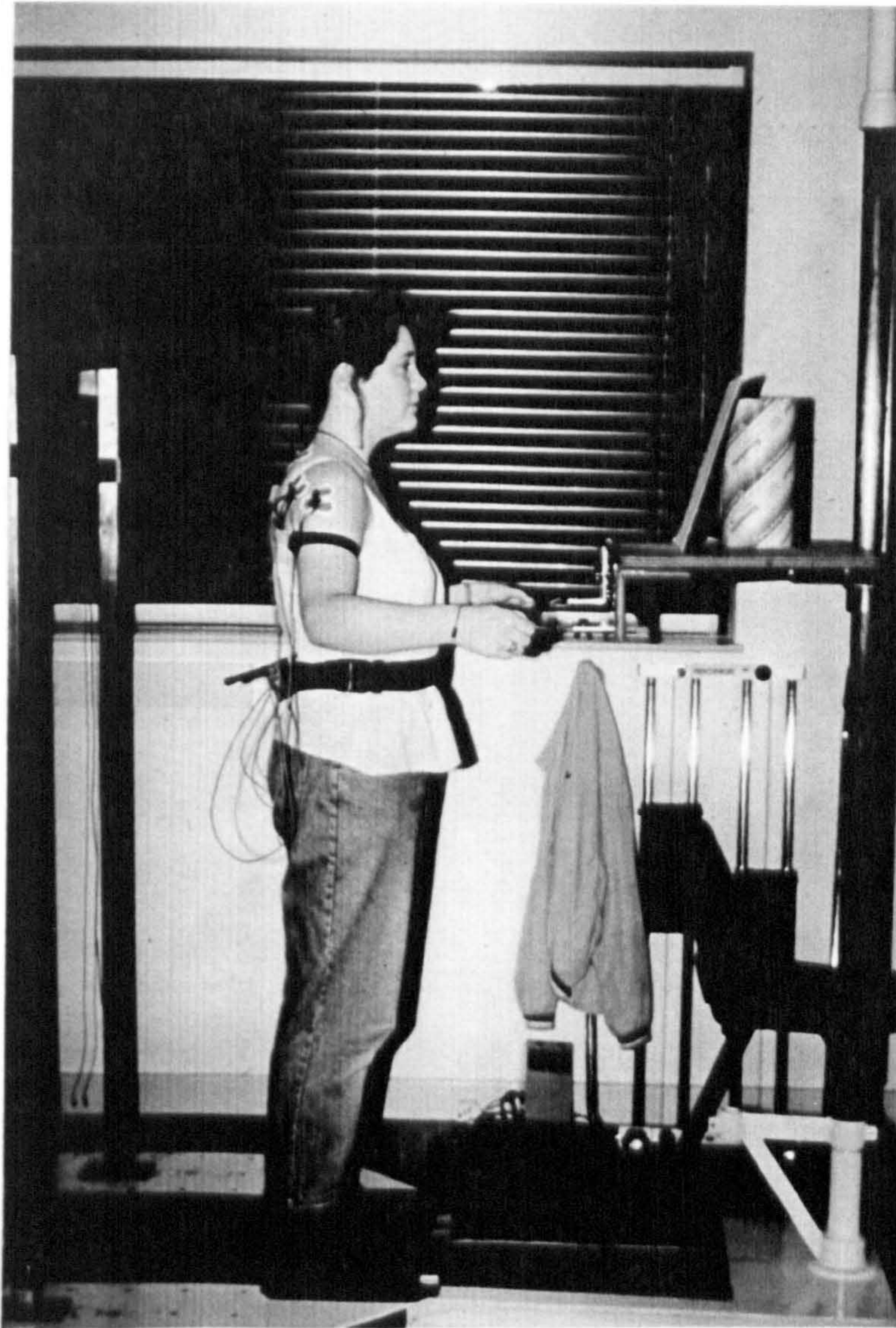
Figure 3.5 Full view of the experimental set-up used during the measurement of maximal endurance to arm abduction. The case illustrated was the holding at 30°.
