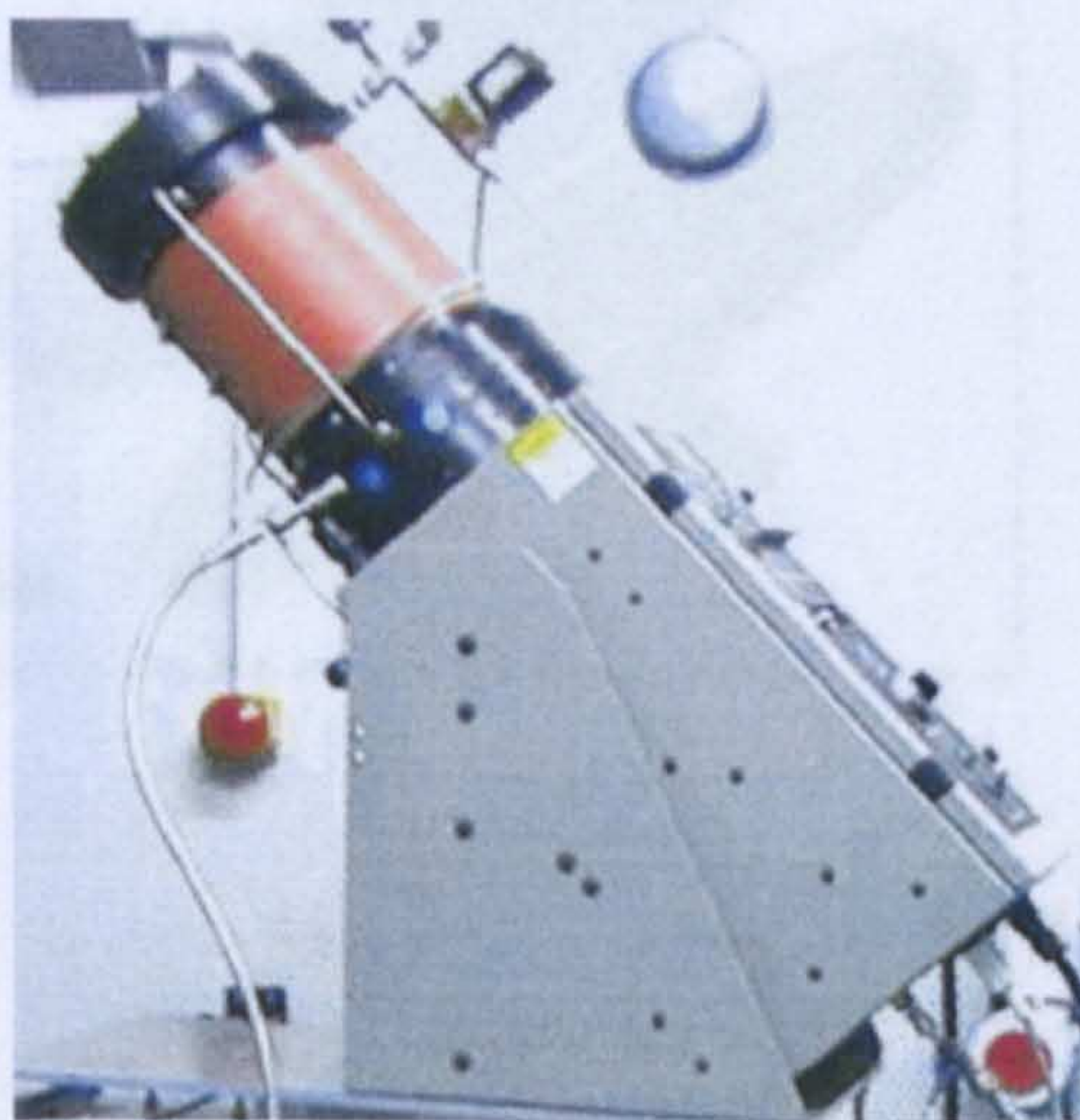
Figure 4.9: Praxair high-pressure powder feeder with the heating jacket.
