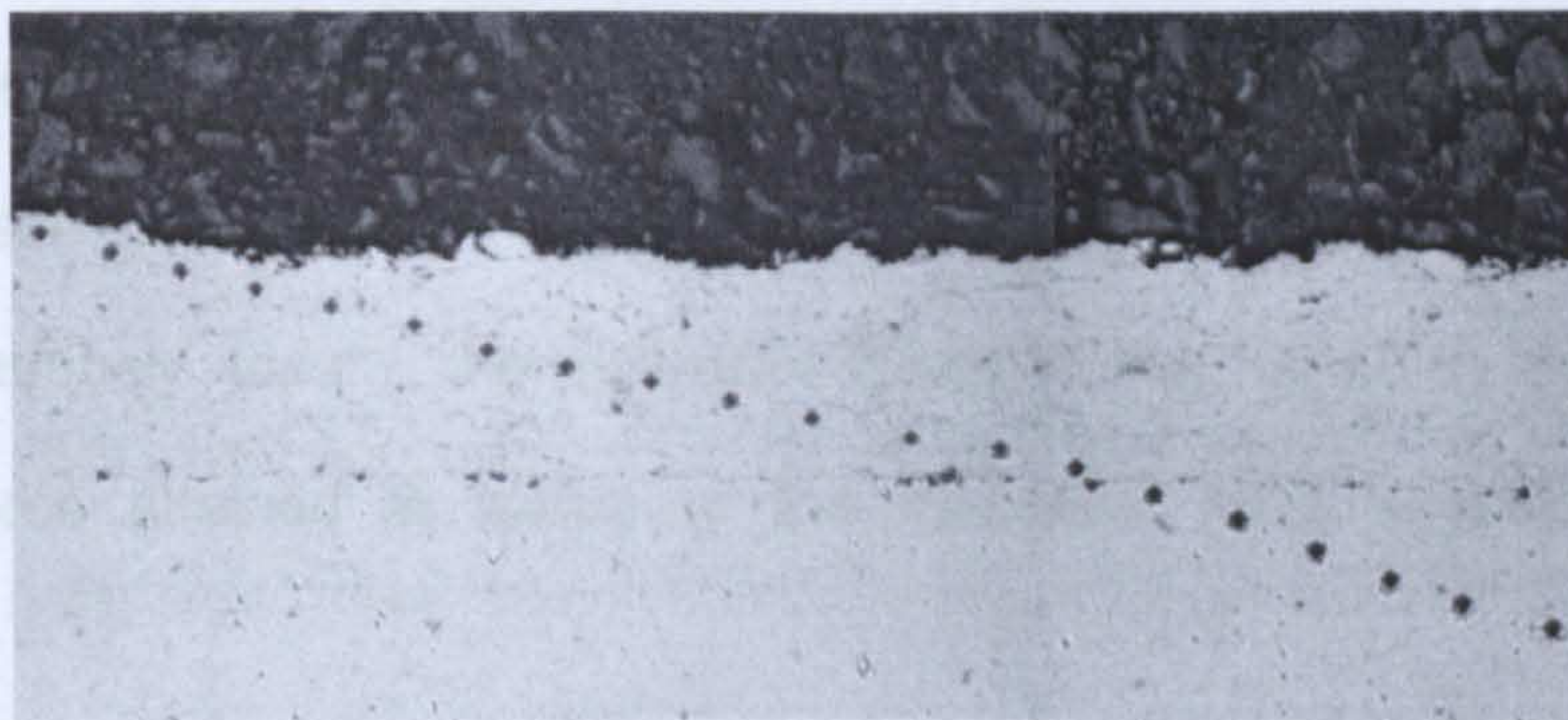
Figure 3.4: Typical microhardness profile on a coating cross-section.
