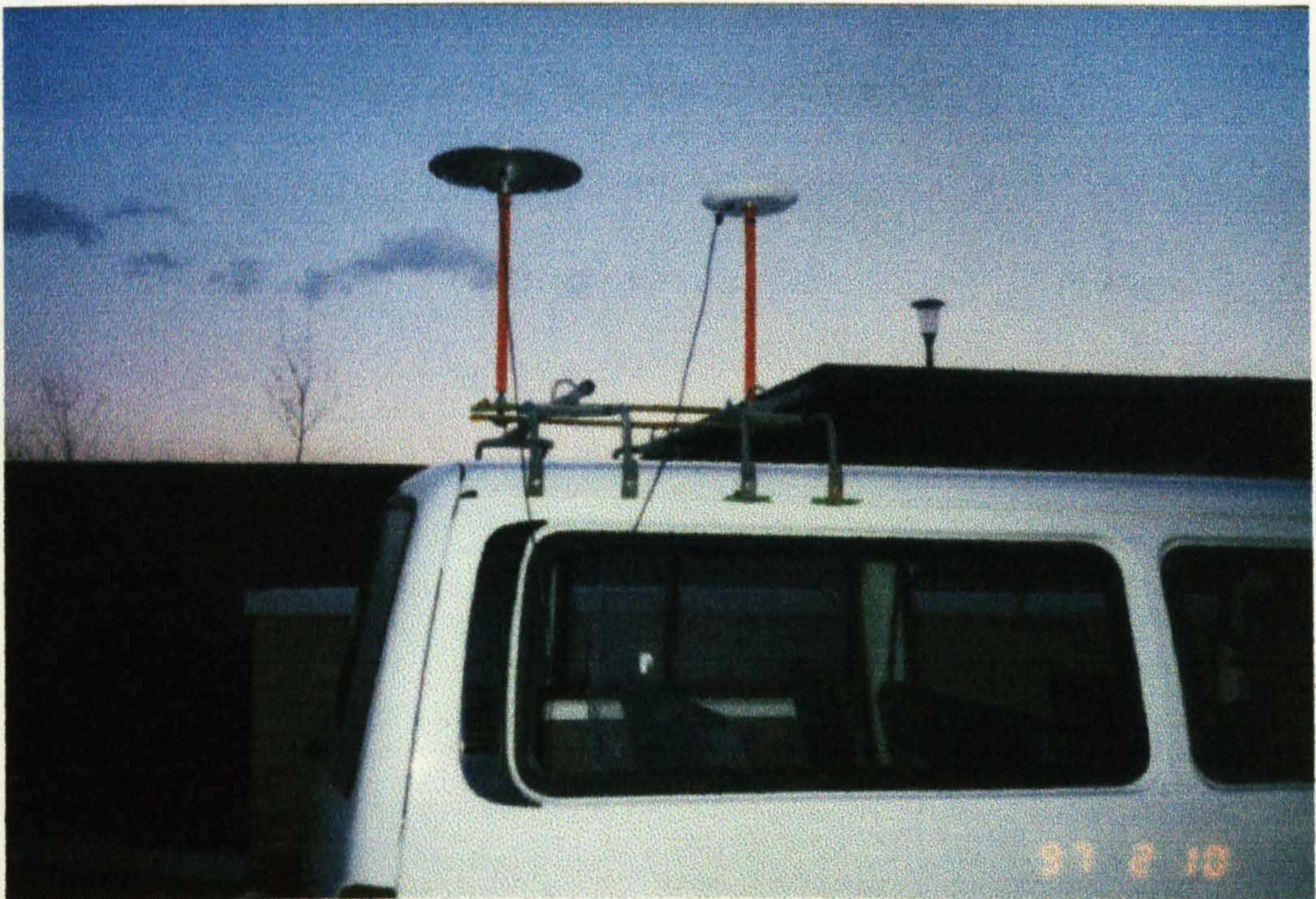
Plate 6.1 Roof Rack, Antenna and Cabling Set-Up
