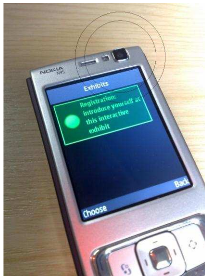
Figure 52 Secondary, front-facing camera type required for full coupled interaction at Registration coupling opportunity
