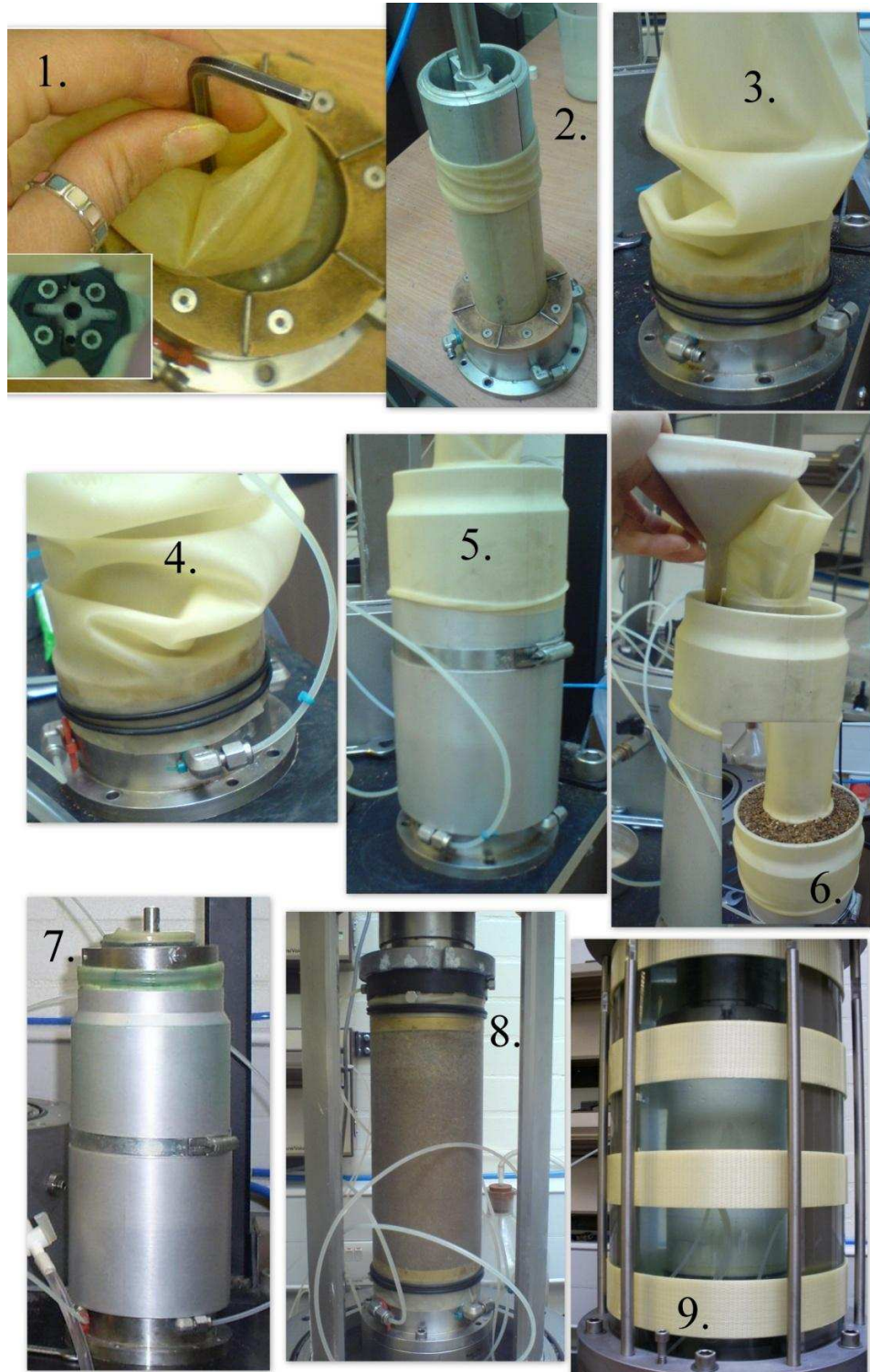
Figure 3-11 Specimen preparation procedures
