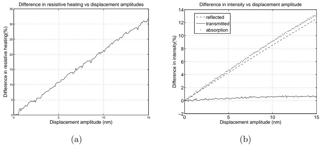
Figure 4.60: (a) The mean time-averaged resistive heating in the d-eCHOT models (extracted from the background film). It can be seen that the resistive heating is increasing with the displacement amplitude, as a percentage of the resistive heating when there is no SAW (when the displacement amplitude is zero). It can be seen that the increase is linear with the displacement amplitude. This demonstrates the contribution of the resistive heating to the device operation (b) The difference in the reflected and the transmitted field intensity of an eCHOT as a percentage of the incident intensity at different displacement amplitudes. The reflected component is essentially twice the signal amplitude, which grows linearly. The transmitted component has a smaller slope. It can be seen that the amount of change in transmission is not big enough to compensate for the increase in the reflected component. This further demonstrates that the absorption/resistive heating is the main operating mechanism in d-eCHOT. Also shown is the calculated absorption from the model. It has a bigger slope than the difference in reflection, since the transmission is out of phase with the absorption.
