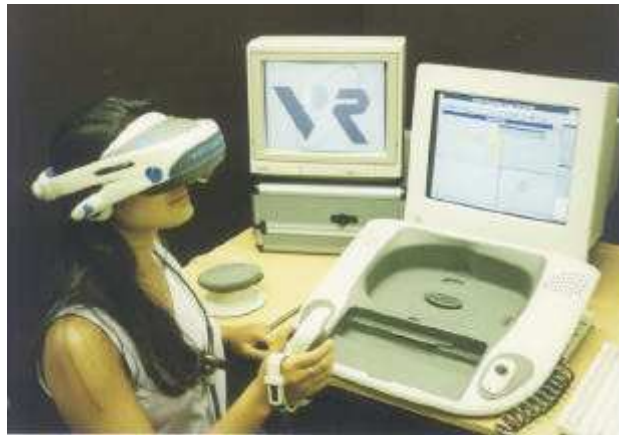
Figure 2.10: An example of Headset system, the Elysium system developed by Virtuality, UK.
