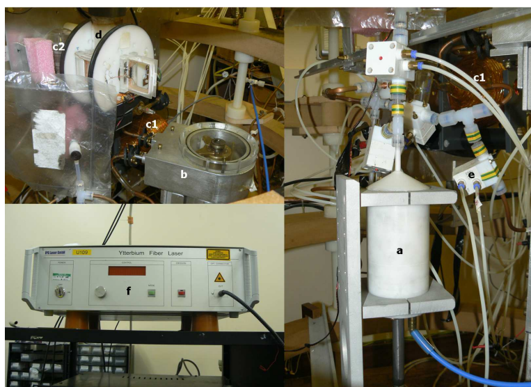
Figure 4.6: A photograph of the final polarisation system indicating the newly added components. a - the cylinder pump used for dispensing the ^3\text{He} b - the peristaltic pump with 4 rollers; c1 and c2 - the new storage cells, c2 is placed next to the optical pumping cell d to allow recording the NMR spectra of both c2 and d ; e - one of the new valves used to control the gas flow; f - the new 20 W Ytterbium fibre laser used to polarise the ^3\text{He} .
