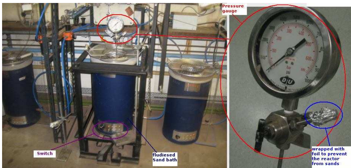
Figure 3.4: Fluidised sand bath and pressure gauge reactor set-up
