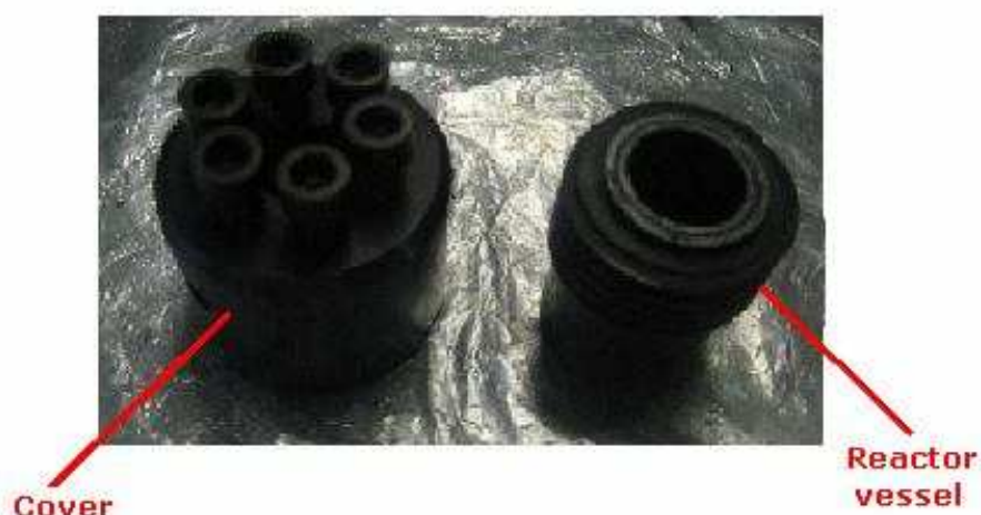
Figure 3.6: Breakdown of pressure gauge reactor (cover & reactor vessel)
