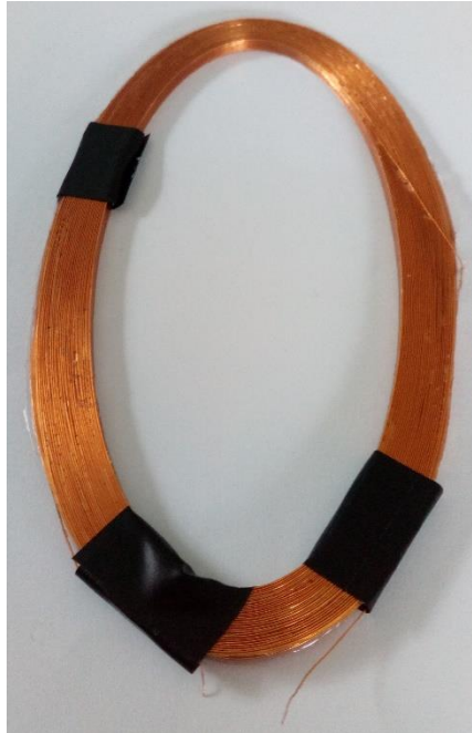
Figure 1.9: One of ESTCube-2 Flight Model elliptical magnetorquers for the long side. Tape protects the loose wire ends from breaking off.
