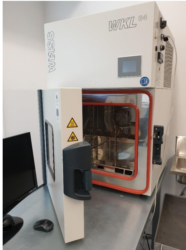
Figure 1.3: Weiss WKL 64/40 Temperature chamber
