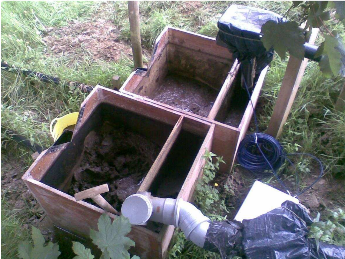
Figure 3.5 Removal of sediment deposited in the box weirs at the experimental pasture (05 June 2008).
