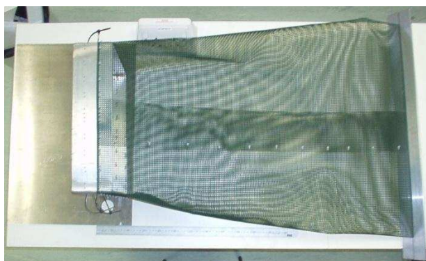
Figure 5.1a-c Bedload traps developed for use on headwater streams in the Pontbren study area. Source of diagram in Figure 5.1a: Bunte et al. (2004); p. 880.
