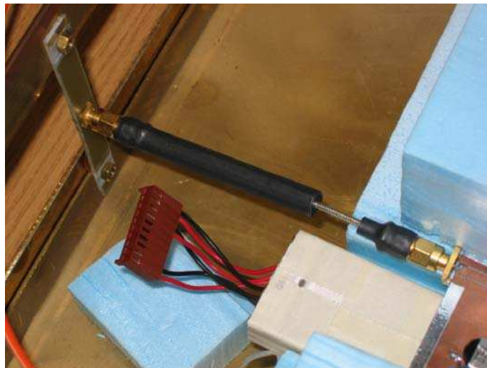
Figure 2.13 The connection from the receiver circuit to the middle of the aperture where the box is excited with a signal
