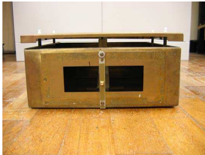
Figure 2.19 Electric and magnetic radiator in an single EUT
