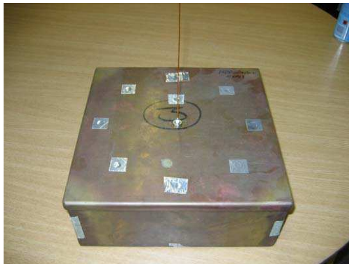
Figure 2.16 A metal box with one monopole on top
