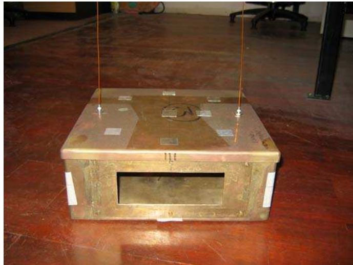
Figure 2.17 A metal box with two monopoles on top
