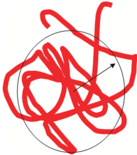
Figure 1.5: A linear polymer molecule chain that is randomly distributed in space. The black arrow shows the gyration radius of it.
