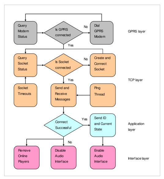
Figure 7-7: Four-Layer communications platform
