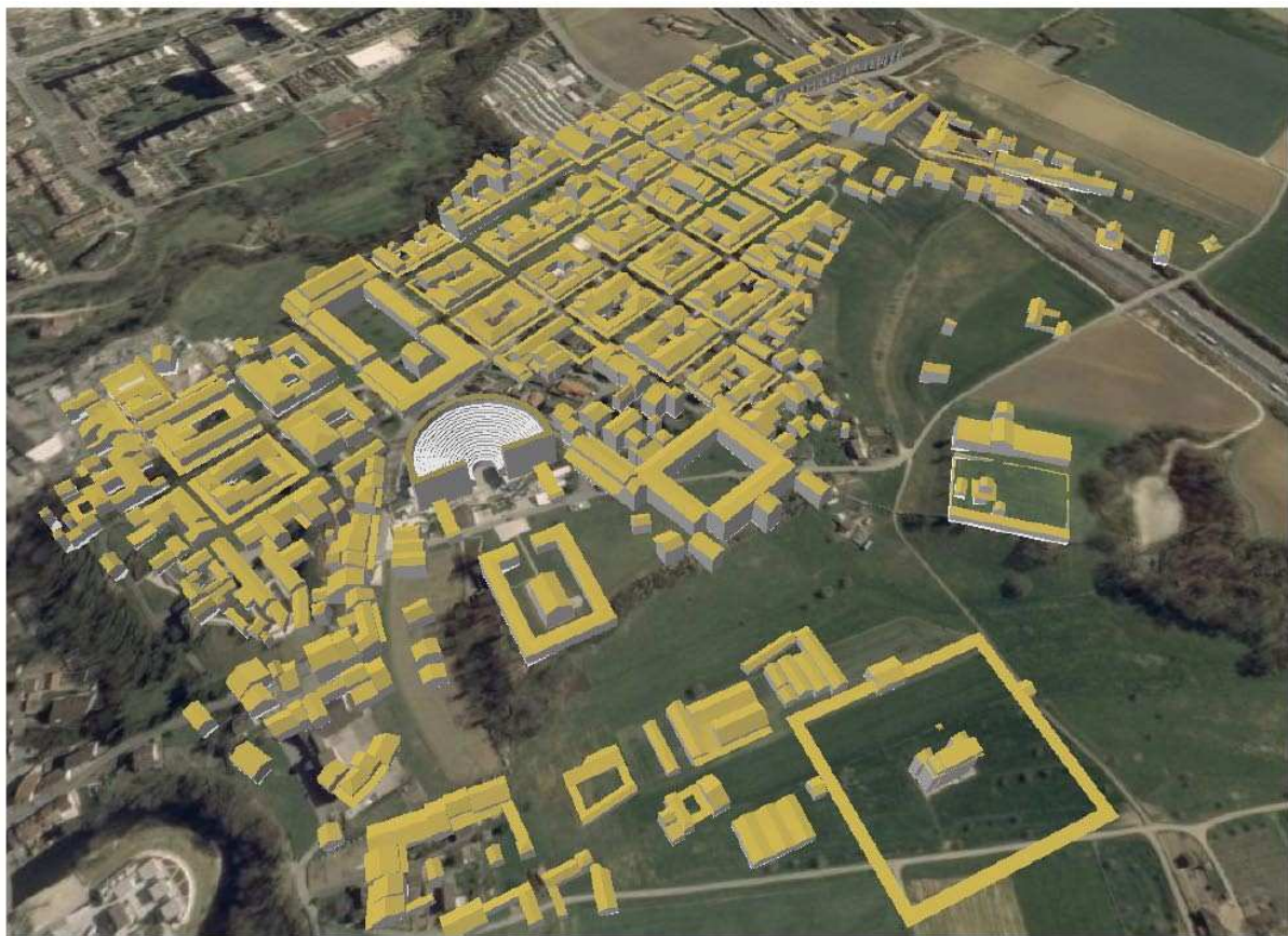
Figure 17 3D city model of the ancient city of Augusta Raurica- Switzerland with modern orthoimages and height model (adapted from Salathé, 2001)
