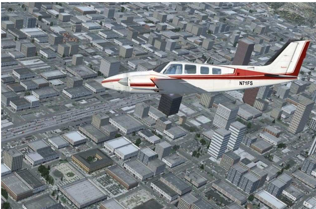
Figure 12 Example of LOD2, 3D city models for flight simulations. (Adapted from PC video game Flight Simulator 2004™, Copyright Microsoft Corporation)
