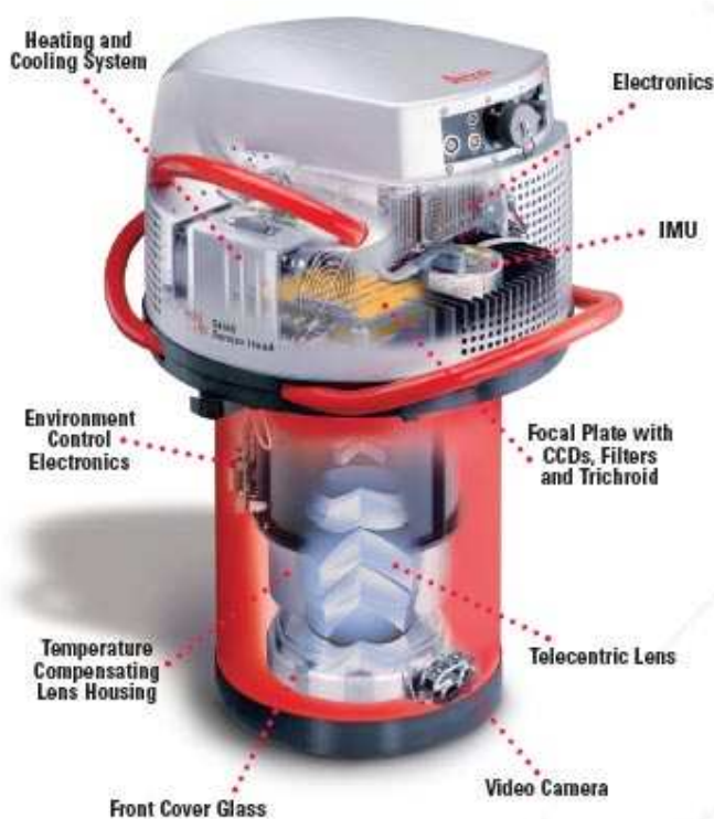
Figure 40 The major components of the ADS40 (ADS40 flyer, 2004)
