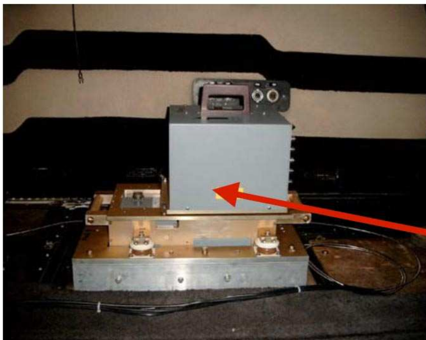
Figure 56 The integrated ALTM sensor with the Applanix DSS camera (adapted from ALTM brochure, 2008)
