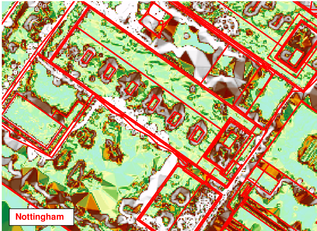
Figure 144 The initial 3D breaklines of the internal roof structures formed when the slope change is greater than 20 degrees.
