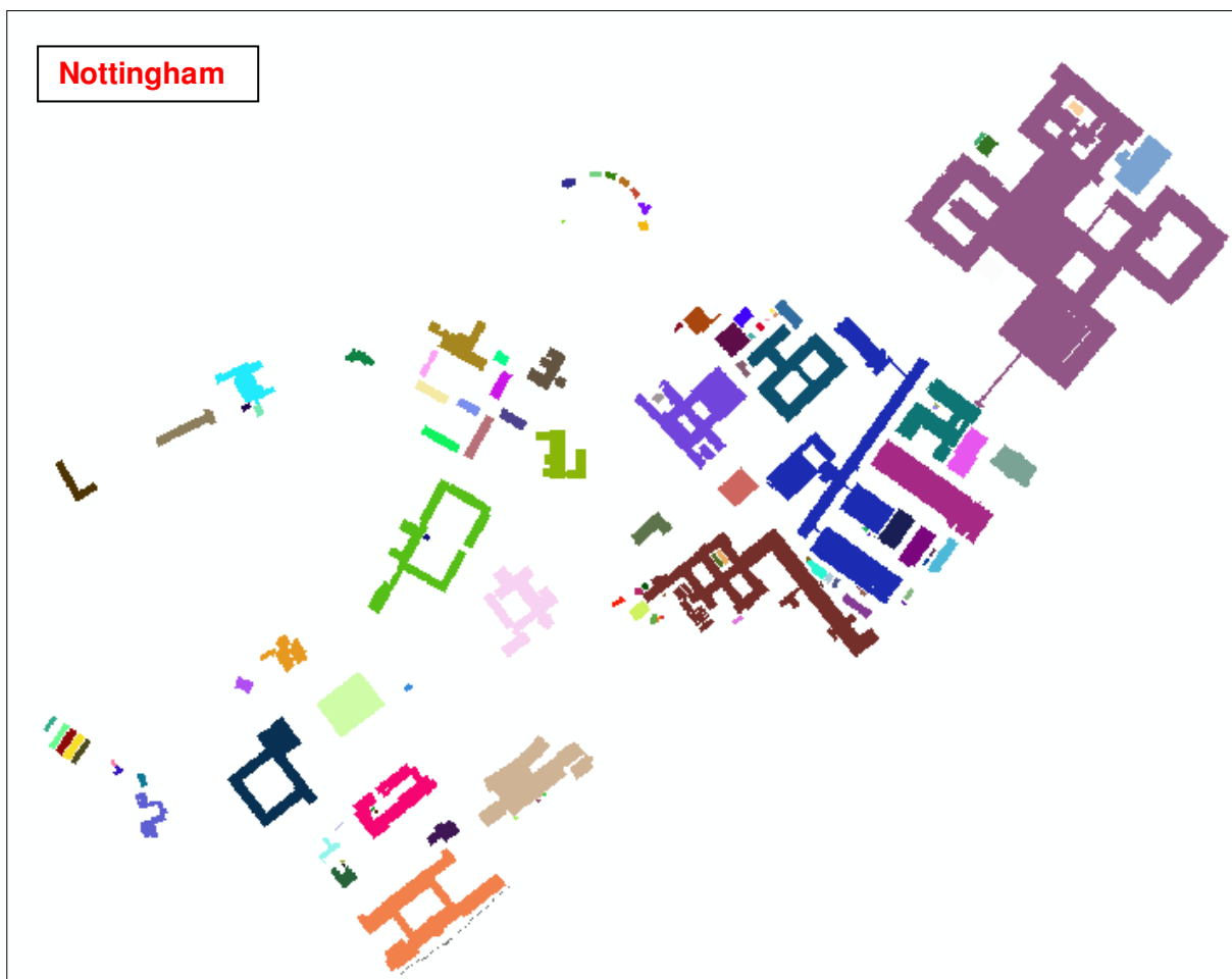
Figure 138 The raster polygons as created from the VDDSM classification process for London and Nottingham. Note each raster building object has been assigned a unique DN value
