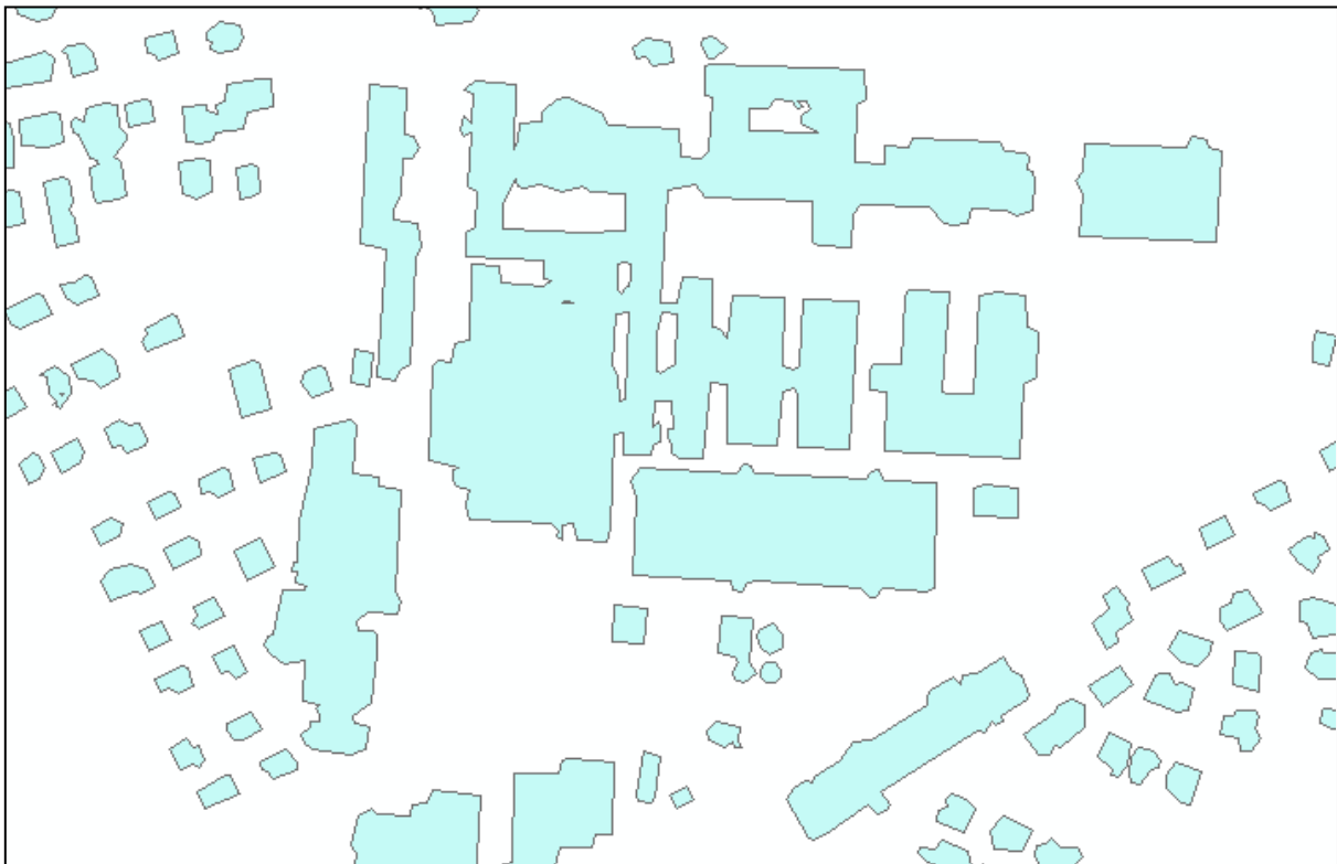
Figure 116 Polygon layer of building hypothesis, produced from the raster to vector conversion process.
