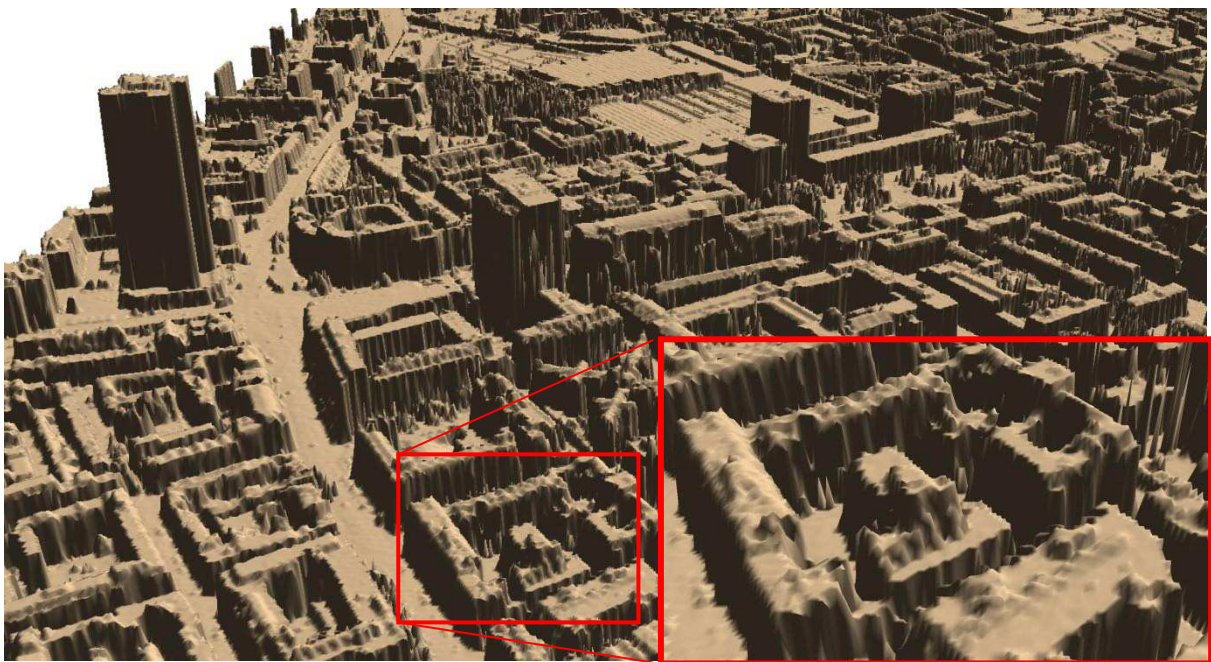
Figure 71 3D perspective scene from the LiDAR data representing the overall density of the surface and highlighting the limitations for adequate representation of roof details.
