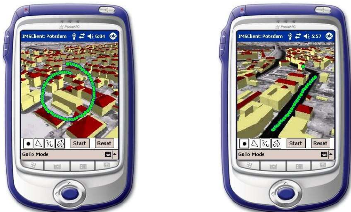
Figure 18 A sketch based navigation system using LOD2 3D city models. Look around the area (left), sketching a navigation command to walk along the street (right). (Adapted from Jurgen et al., 2005)
