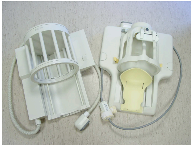
Figure 2.26: Philips' T/R (left) and 8-channel SENSE (right) RF coils.
